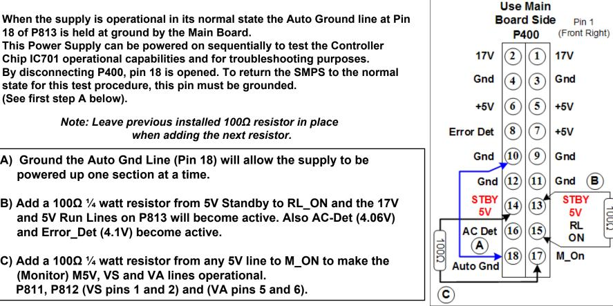
This Power Supply can be powered on sequentially to test the Controller Chip IC701 operational capabilities and for troubleshooting purposes. By disconnecting P400, pin 18 is opened. To return the SMPS to the normal state for this test procedure, this pin must be grounded. (See first step A below).
