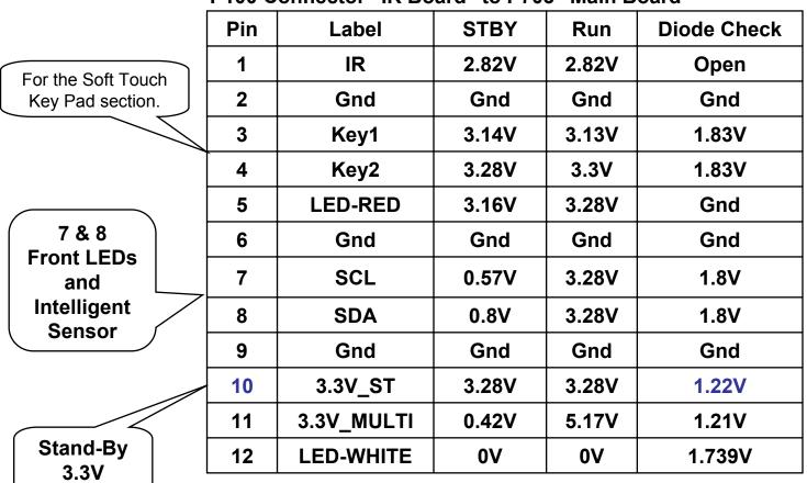
P100 Connector "IR Board" to P703 "Main Board"
