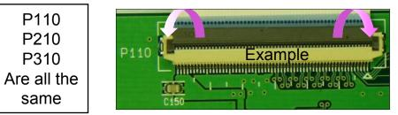
Remove tape (if present) and <u>Gently</u> pry the locking mechanism upward and remove the ribbon cable from the connector.
