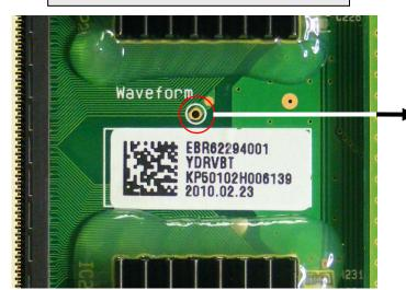
NOTE: The Waveform Test Points are fragile. If by accident the land is torn and the run lifted, make sure there are no lines left to right in the screen picture.
