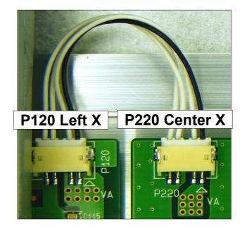
Va Right 2 pins Gnd Left 2 pins
