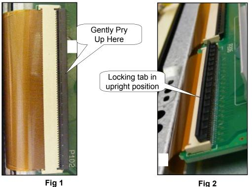
Be sure ribbon tab is released By lifting the ribbon up slightly, before removing ribbon.
