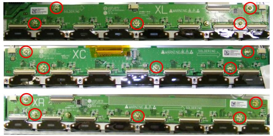
The Left X Board passes drive signals to 8 TCP's on the right side of the screen The Center X Board passes drive signals to 7 TCP's in the center of the screen The Right X Board passes drive signals to 8 TCP's on left side of the screen
