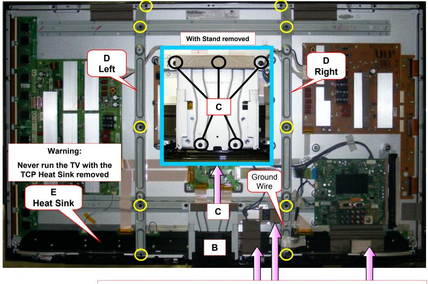
Warning Shorting Hazard: Conductive Tape. Do not allow to touch energized circuits.
