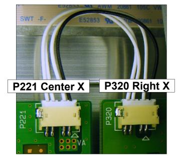
Va Right 2 pins Gnd Left 2 pins Both Connectors
