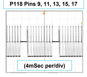
The signal for these pins look very similar due to the fact they are read from Chassis Gnd, but they are actually Floating Ground related. DO NOT hook scope Gnd to Floating Gnd TP without an Isolation Transformer.
