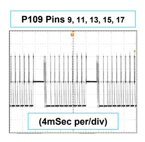
The signal for these pins look very similar due to the fact they are read from Chassis Gnd, but they are actually Floating Ground related. DO NOT hook scope Gnd to Floating Gnd TP without an Isolation Transformer.
