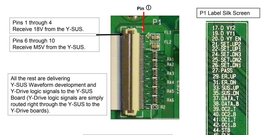
Note: The +18V is not used by the Control board, it is routed to the Z-SUS leaving on P2 Pins 14~15.
