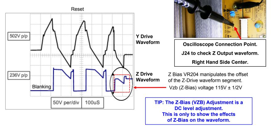
This Waveform is just for reference to observe the effects of Z Bias adjustment
