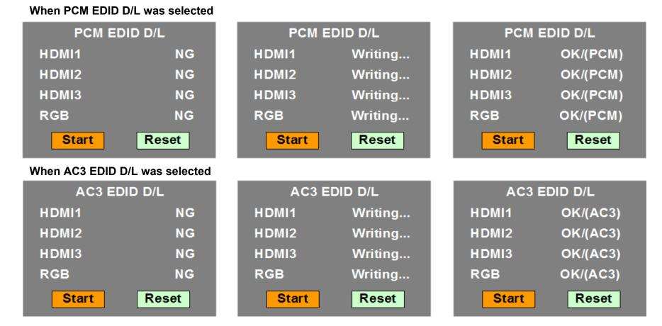
Note: When PCM is downloaded, AC3 will be N/G and when AC3 is downloaded PCM will be N/G. This means that when PCM is OK, PCM audio is priority and when AC3 is OK, AC3 audio is priority.
