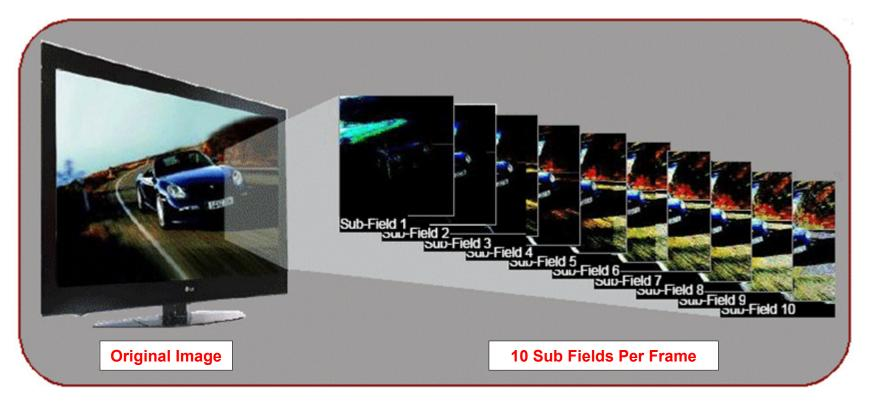
Sub Field firing occurs using wall charge and polarity differences between Y-SUS and Z-SUS signals.
