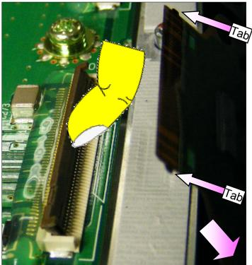
The TCP Ribbon Cable has two small tabs on each side which help secure it into the connector. They have to be lifted up slightly to pull the Ribbon Cable out. Note: TCP is usually stuck down to the Chocolate heat transfer material, be Very Careful when lifting up on the TCP ribbon cable.
