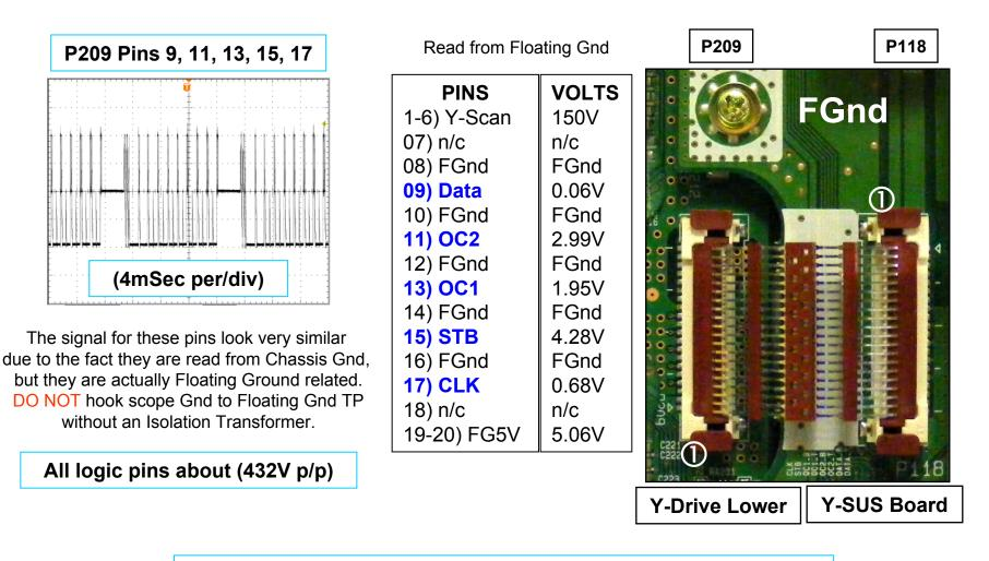
P209 Pins 9, 11, 13, 15, 17 are Logic (Drive) Signals to the Y-Drive Lower.
