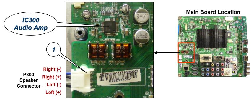
Diode Mode Check with the Board Disconnected. DVM in the Diode mode.
