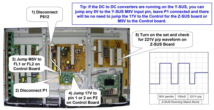
The Power Supply should be producing 17V or you can substitute voltage matching 17V from an external source to either pins 1 or 2 on connector P2 on the Control board.
