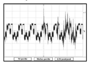
Example of Normal Signals measured at 1V p/p at 10µSec
