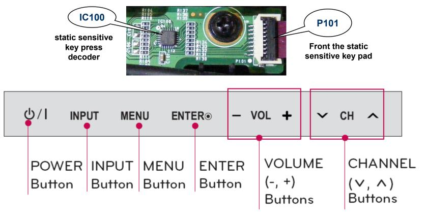
Button Identification for the Front the static sensitive key pad
