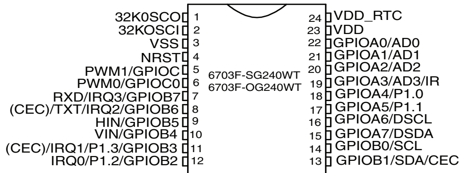
Figure 8-2 Internal block diagram and Pin configuration
