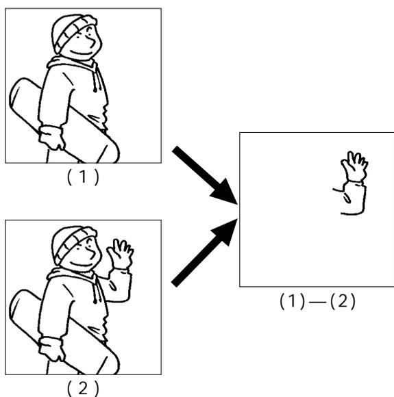
1. Pictures (1) and (2) to be reproduced as time elapses have many elements common to each other. Differential or (1) minus (2) is extracted and (2) is reproduced by synthesizing the differential with (1).
