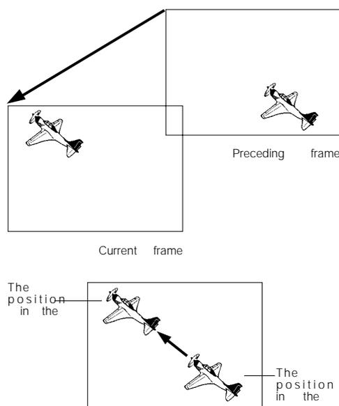
2. In the motion compensation process, pictures are divided into blocks and the motion vector which indicates the amount of movement is extracted and coded for the part whose position changes, without changing its shape. By combining this motion compensation with predictive coding, data is more efficiently compressed.
