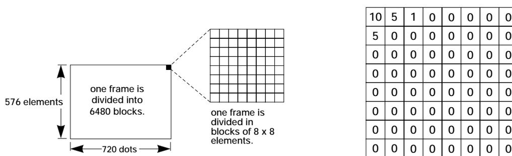
Changes in luminance and color are small in some parts of a frame (low frequency) while changes are large in other parts (high frequency) and a frame can be considered as an overlaid composite picture comprised of a very low frequency picture, a low frequency picture, a high frequency picture, and a very high frequency picture.
