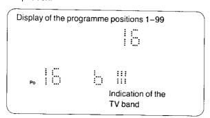
The tuner in the VTR can be preset with up to 99 stations.
