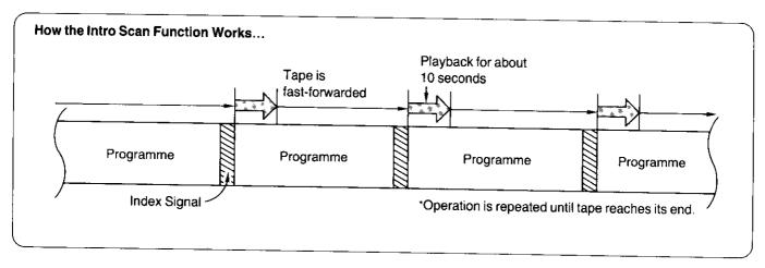
The Intro Scan function plays back the first 10 seconds of each programme (recorded with index signal) on a tape one after another. This is convenient for quick checking what programmes are on a tape, or to find the desired instalment of a TV series you have recorded on a tape.
