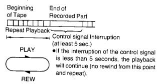
3 To stop the Repeat playback, press either the Stop Button or the Memory/Repeat/Search Button (the Repeat Indicator "R" will go out.)
