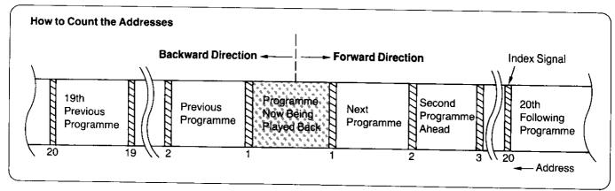
With the VHS Index Search function, up to 20 addresses (places where index signals are recorded) can be skipped to directly locate the beginning of the desired programme in both forward and reverse direction in the Fast Forward or Rewind mode.
