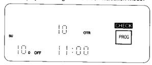
The VTR will automatically switch off, when the OTR is completed. To turn the VTR on again, press the VTR On/Off Switch.
