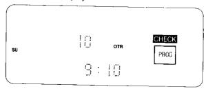
When the Clock/Counter Selector Button (Remote Controller) is pressed during OTR recording, the display will change over to the counter mode.
