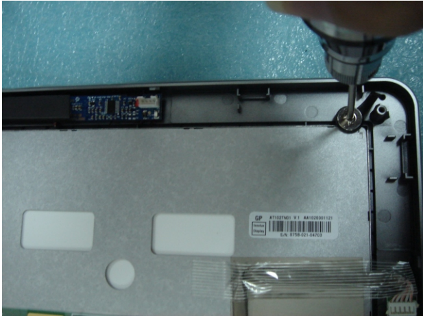
11. Disassemble display screen and other subsidiary board after remove flat cable.
