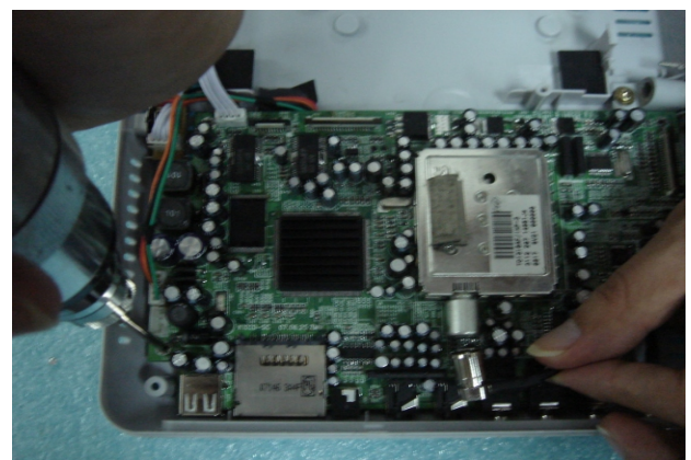
15. Take out main board screw and take out video main board.
