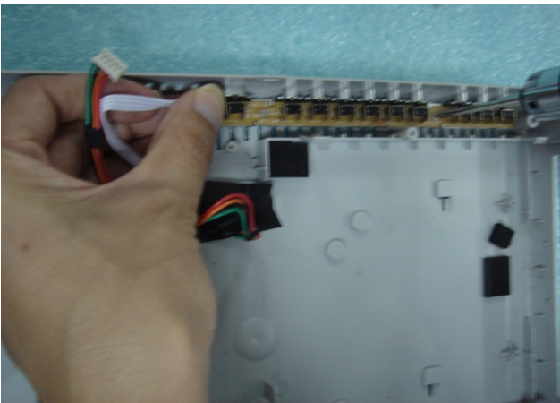
1. Install buttonboard/battery socket/antenna extending wire to bottom casing without scrap bottom casing.
