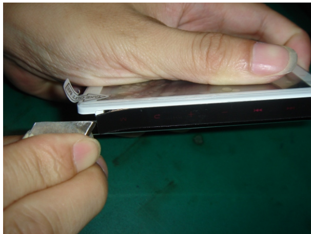
2. Use blade to remove the glass from the gap on one side of the glass.
