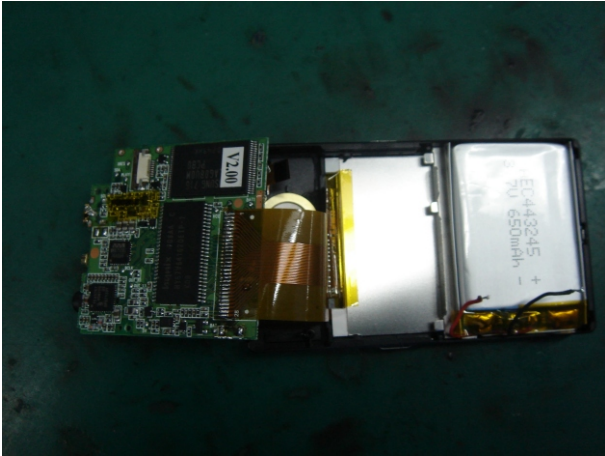
11. Take out battery components.
