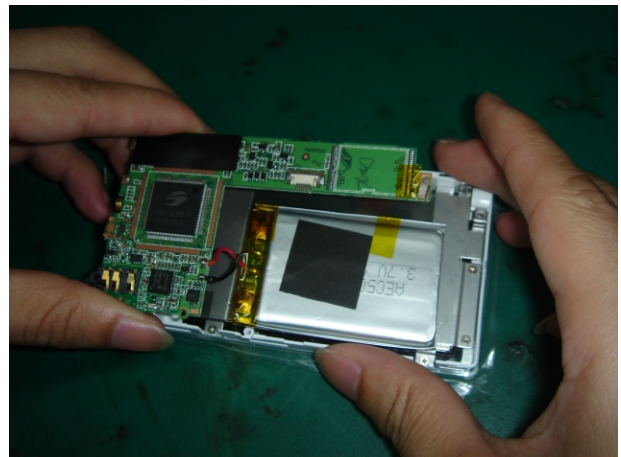
8. Take out the main board from middle casing.
