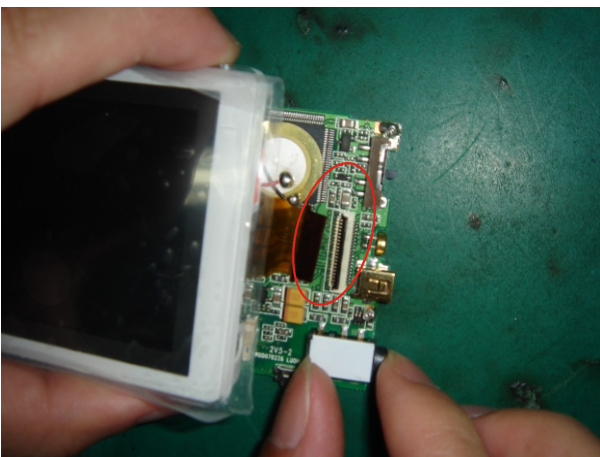
9. Use forceps to pull out display screen flat cable and then take out main board.
