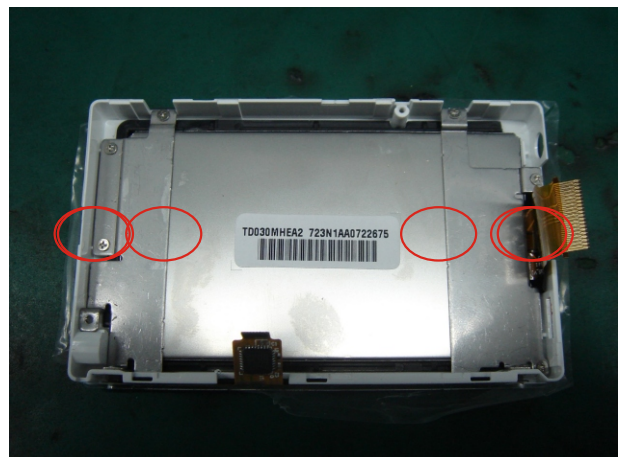
10. Use electric screwdriver or "+"-shaped screwdriver to take out 6 screws of cover board, take out display screen cover board and then the display screen components.
