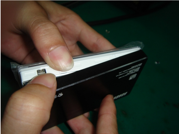
5. Separate the bottom casing and the middle casing.
