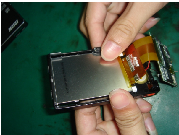
13. Take out display screen components from the direction shown in the picture
