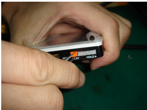
1. Use cuspidal forceps to take out the LOCK button;
