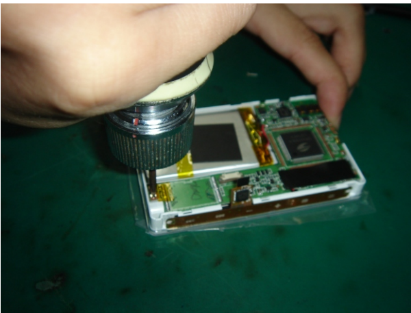
7. Take out 2 screws of main board.
