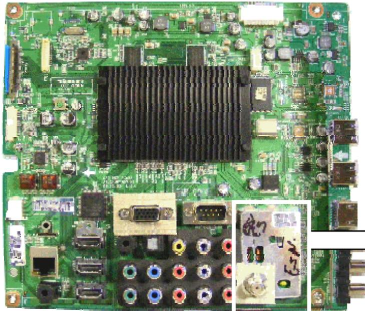
To keep the Data and Clock lines running so they can be measured easily, place the unit into "Auto Tuning".
