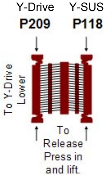
**This connector does not come with a new Y-SUS or Y-Drive.**
