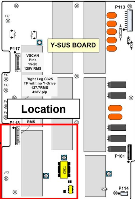
**FG5V (Floating Ground 5V). Checked at IC304 Left Leg.**
