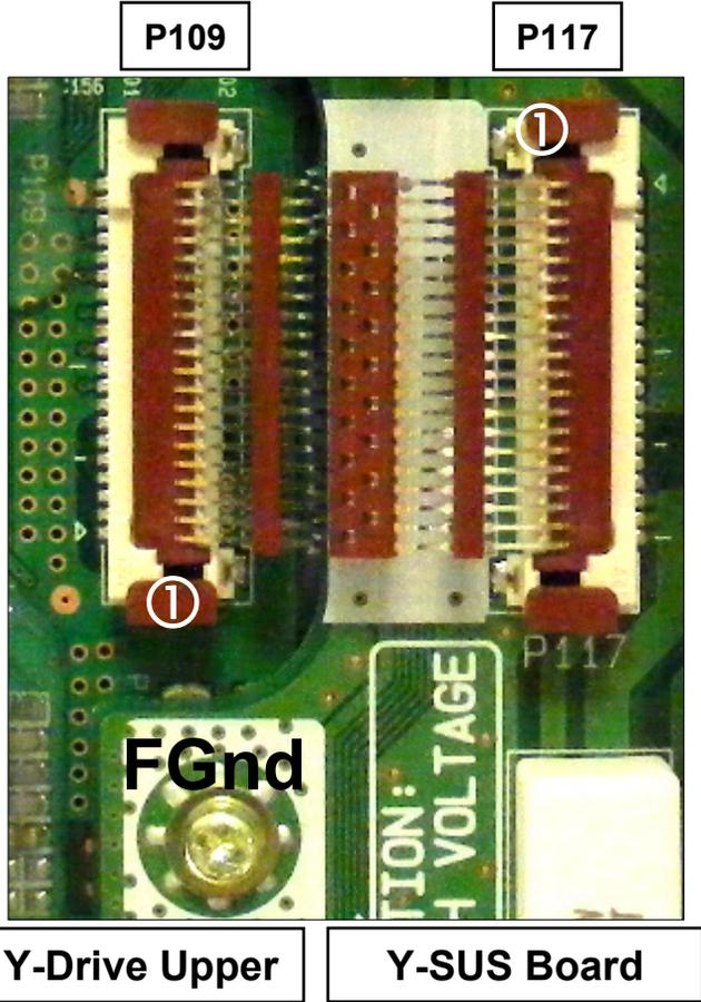
**P109 Pins 9, 11, 13, 15, 17 are Logic (Drive) Signals to the Y-Drive Upper.**
