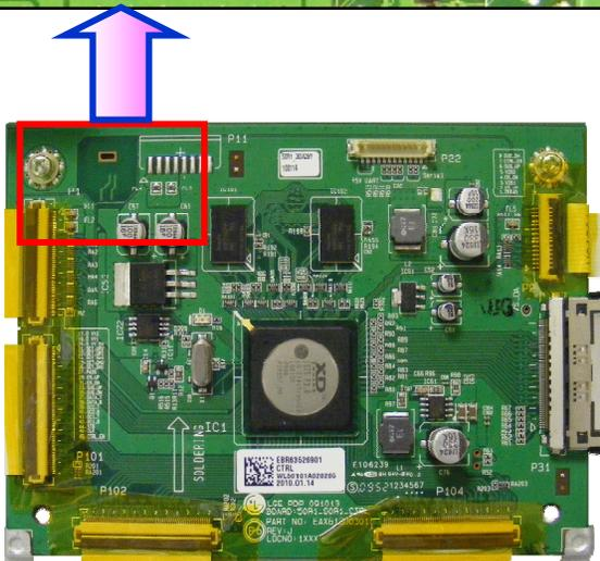
**CONTROL BOARD TEMPERATURE SENSOR LOCATION**
