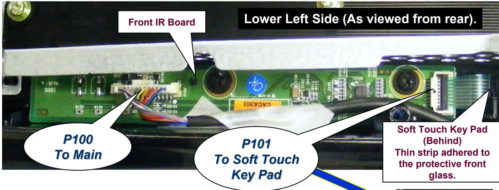
To remove P101 ribbon, using your fingernail, lift up the locking mechanism. Slide the board out to the left to release the ribbon cable.
