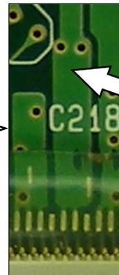
All Connectors to All TCPs look very similar for the 3.3V test point. The trace at pins 33 and 34 of each connector. There will be two small feed troughs, (TP) you can use for Test Points. Example here from P203. You can only check for continuity back to IC53, you can not run the set with heat sink removed.
