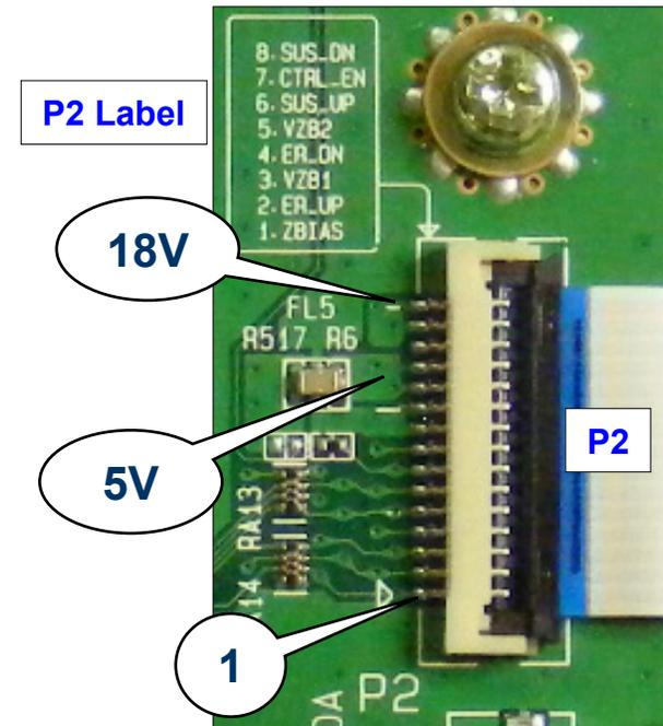
Diode Mode Readings taken with all connectors Disconnected. Black lead on Gnd. DVM in Diode Mode.
