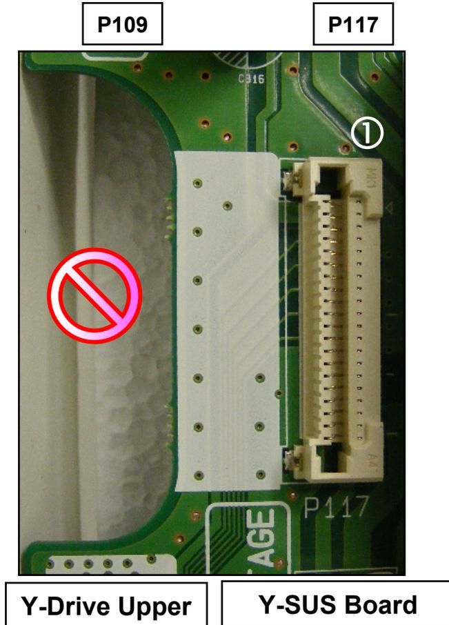
Y-Drive Board should be disconnected for this test.
