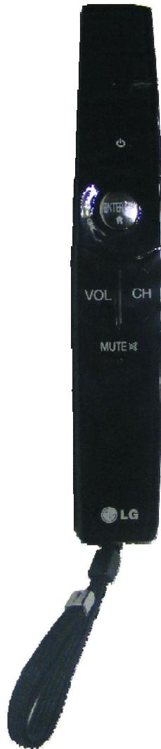
The first time the Motion Remote has its batteries installed and pointed at the Television, the Motion Remote is synchronized with the TV. After that, when pointing the remote at the TV and pressing the Enter key, a pointer appears on screen, then by moving the Motion Remote around, the pointer moves with the movement of the remote. When the pointer is placed over a selectable button, you can press the center “Enter” button and activate the object. This makes navigation much easier.
