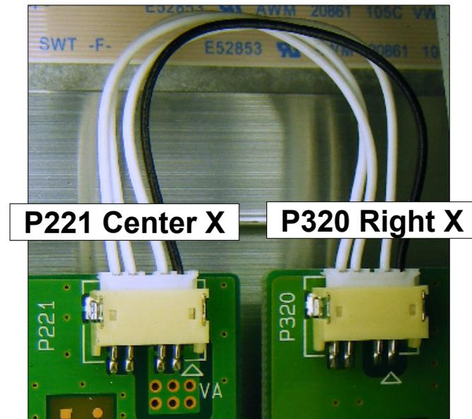
Diode Mode Readings taken with all connectors Disconnected. Black lead on Gnd. DVM in Diode Mode.
