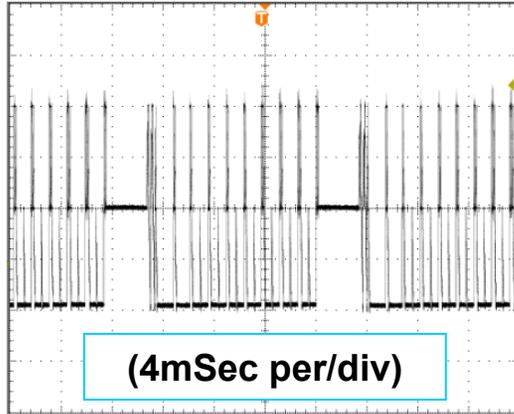
The signal for these pins look very similar due to the fact they are read from Chassis Gnd, but they are actually Floating Ground related. **DO NOT** hook scope Gnd to Floating Gnd TP without an Isolation Transformer.
