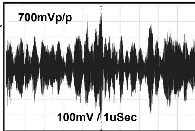
Note: Pin 17 and Pin 18 "Dig IF" Signal 8VSB or QAM Only when receiving a Digital Channel.
