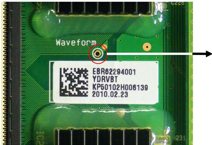
**NOTE: The Waveform Test Points are fragile. If by accident the land is torn and the run lifted, make sure there are no lines left to right in the screen picture.**
