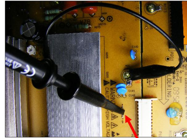
**Oscilloscope Connection Point.
