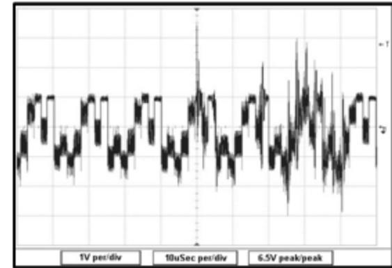
Example of Normal Signals measured at 1V p/p at 10 $\mu$ Sec
