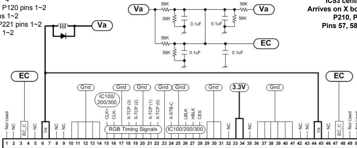
Flexible Printed Ribbon Cable to TCP IC
