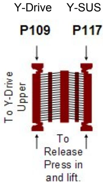
**Warning: Never run the Y-SUS with just P109 disconnected. You must remove the Upper Y-Drive board completely due to these FG lugs.**
