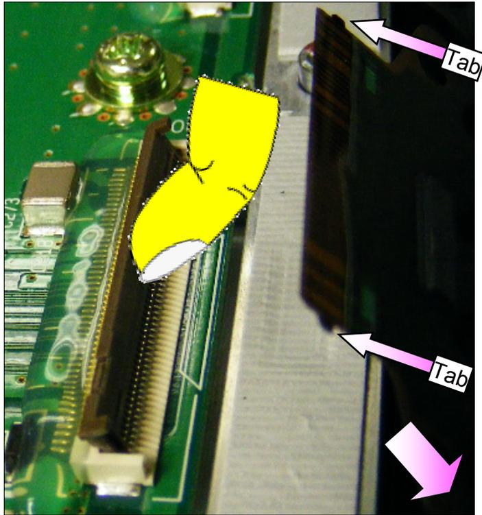
Lift up the locking mechanism as shown to release the ribbon cable.
