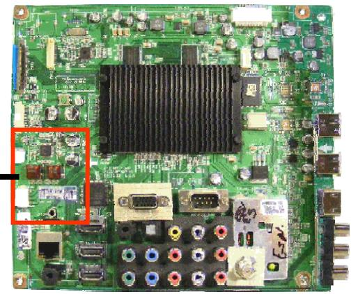
Diode Mode Check with the Board Disconnected. DVM in the Diode mode.
