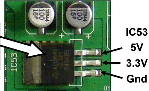
3.3V in on Pins 57 ~ 60 on any connector from the Control board
