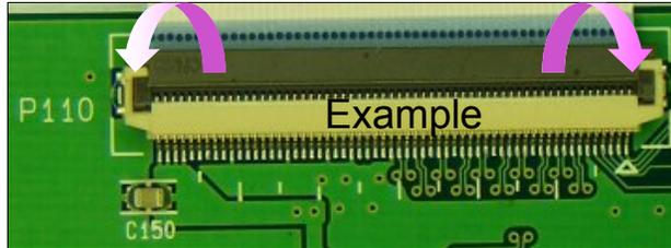
Remove tape (if present) and Gently pry the locking mechanism upward and remove the ribbon cable from the connector.
