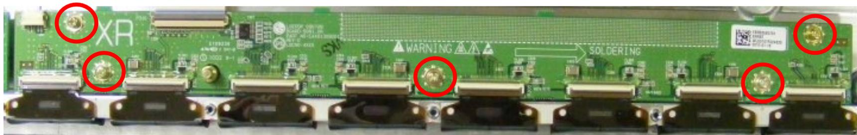
The Left X Board passes drive signals to 8 TCP's on the right side of the screen
