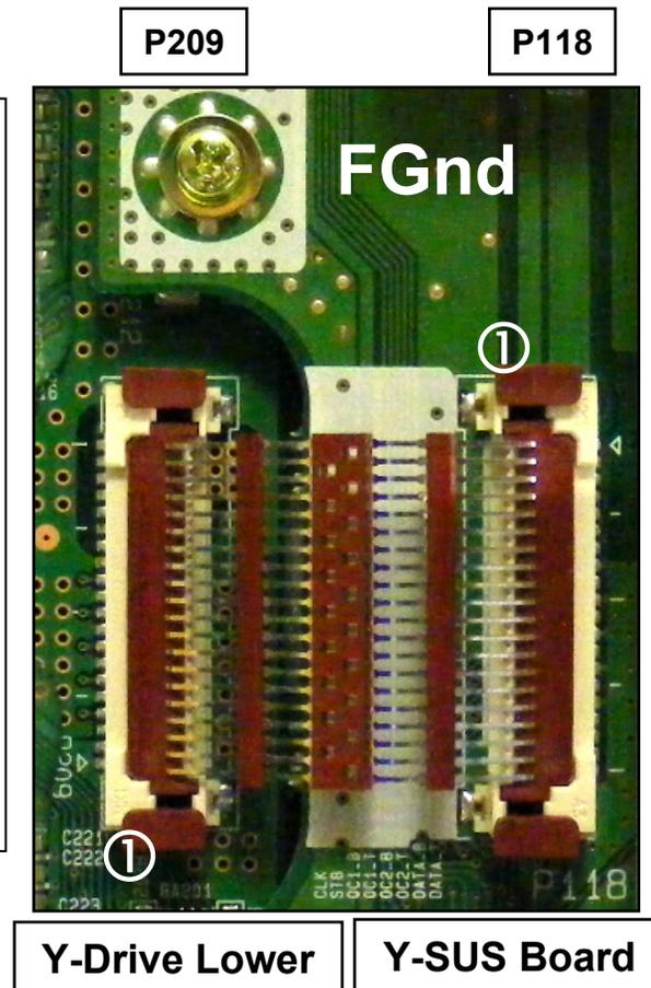
**P209 Pins 9, 11, 13, 15, 17 are Logic (Drive) Signals to the Y-Drive Lower.**
