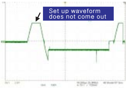
<Fig. 2 When the Pass Set_Up FET is damaged>
