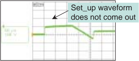
<When the Set_Up FET is damaged>
