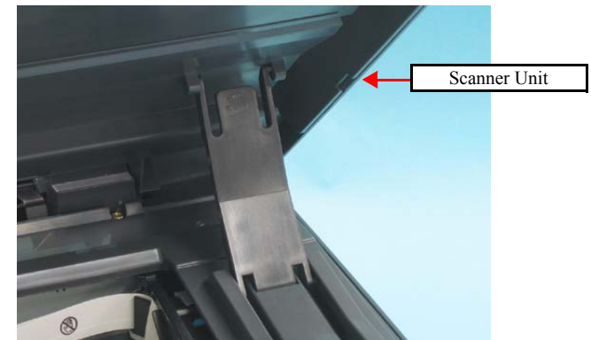
Figure 4-8. Installing Support Arm
