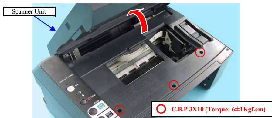
Figure 4-9. Removing Screws securing Middle Case (front side)
