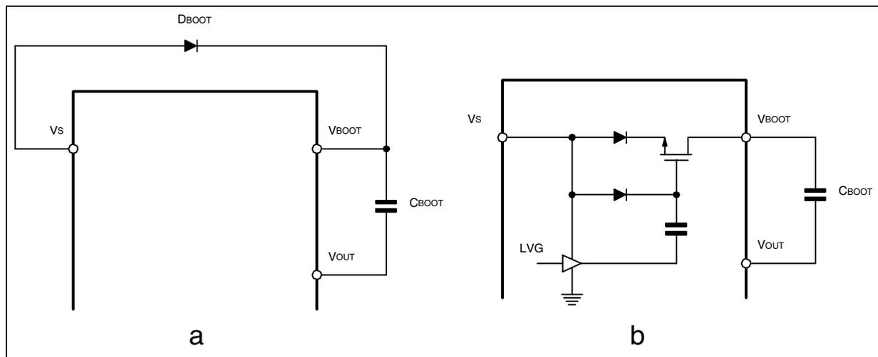
To drive the synchronised DMOS it is necessary a voltage higher than the supply voltage  $V_S$ . This voltage is obtained by means of an internal charge pump (fig. 11b).
