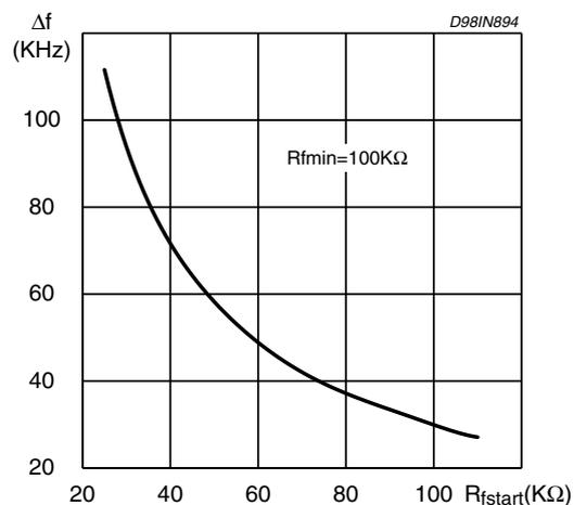
Figure 7. Typ.  $(f_{start}-f_{min})$  vs.  $R_{fstar}$  @  $C_f = 470pF$
