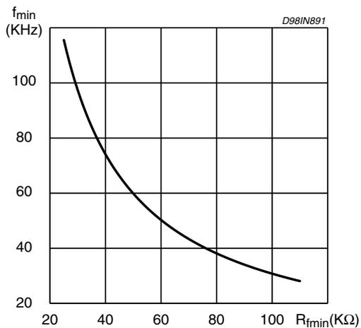
Figure 9. Typ.  $(f_{start}-f_{min})$  vs.  $R_{fstar}$  @  $C_f = 470pF$
