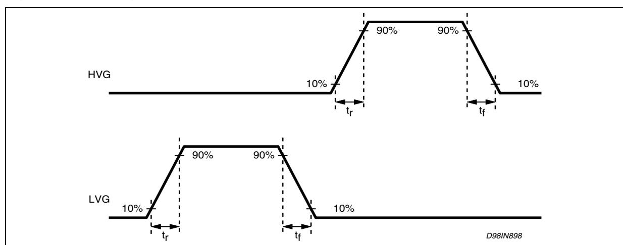
**Figure 13. Dead Time and Duty Cycle Waveform Definition**
