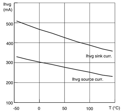
**Figure 20. LVG Source and Sink Current vs. Temperature**
