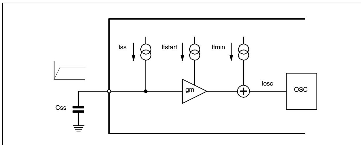
During the soft start time the current  $I_{SS}$  charges the capacitor  $C_{SS}$ , generating a voltage ramp which is delivered to a transconductance amplifier, as shown in fig. 4. Thus this voltage signal is converted in a growing current which is subtracted to  $I_{fstart}$ . Therefore the current which drives the oscillator to set the frequency during the soft start is equal to:
