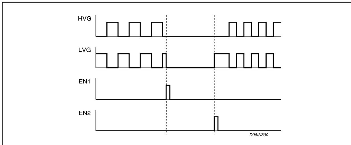
Figure 3. Oscillator/Output Timing Diagram
