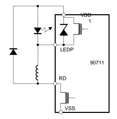
The type of relay should be normally closed (NC). A NC relay is opened by applying the control voltage on its coil and in this case the module is in Auto Shut-Off mode.
