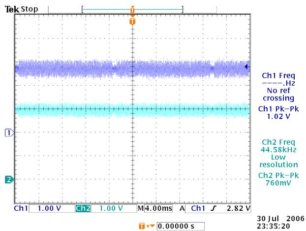
CH1 HDMIMCLK (U19 PIN 79) ;CH2 HDMIBCLK (U19 PIN 76)
