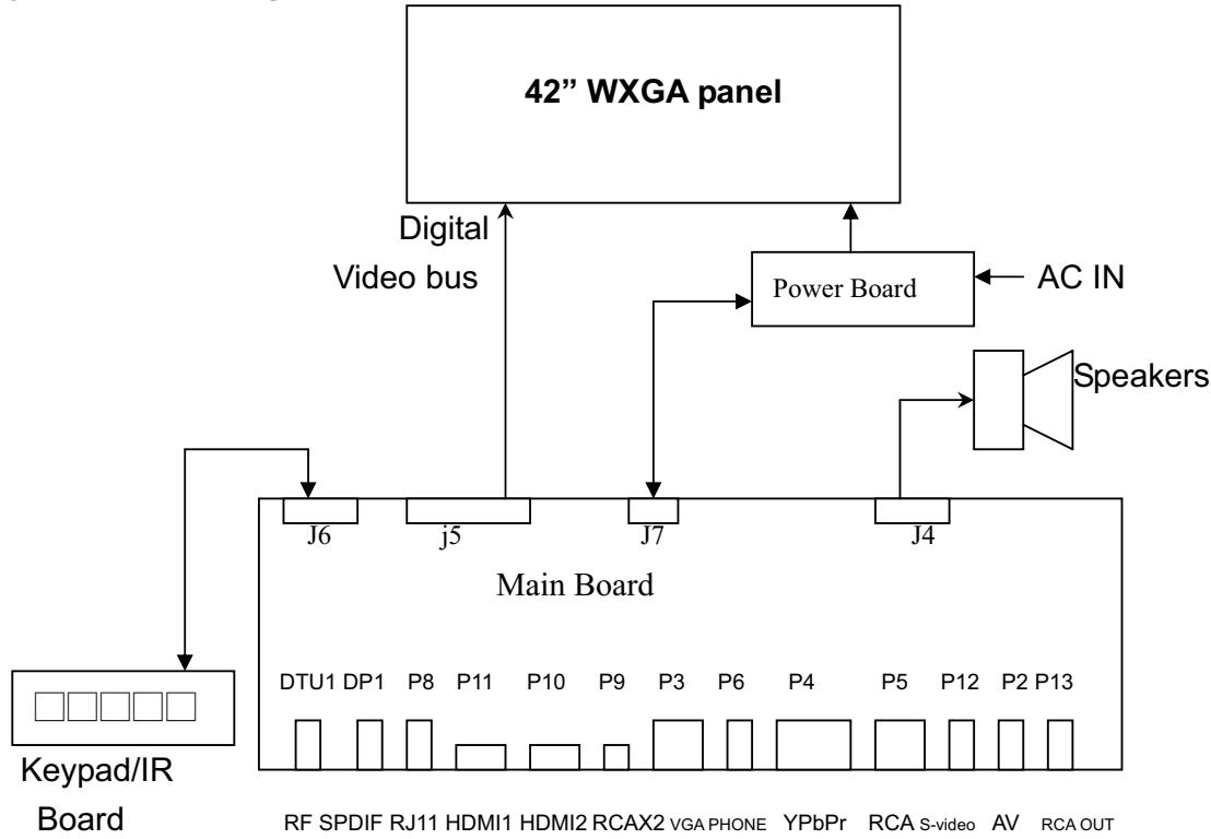
The TV system block diagram is powered by power board that transforms AC source of 100V~240V AC +/- 10% @ 50/60 HZ into DC 5V & 12V& 24Vsource. The main board receives different types of video signal into the MTK8202 Ic. Afterward, the MTK8202 Ic process the signals control the various functions of the monitor and outputs control signal, video signal and power to the 42" WXGA panel to be displayed.
