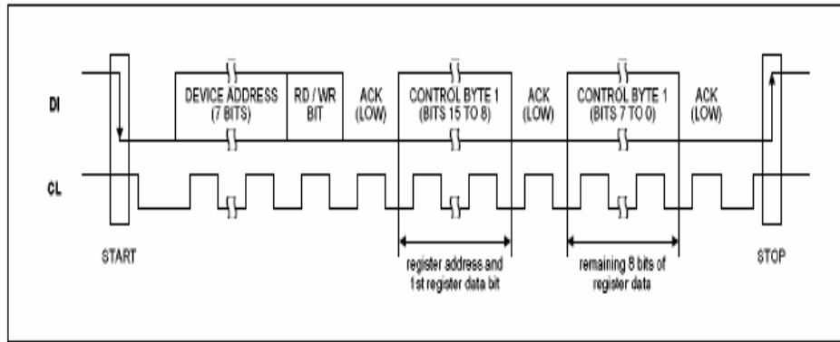
The wm8776 has two possible device addresses, which can be selected using the CE pin
