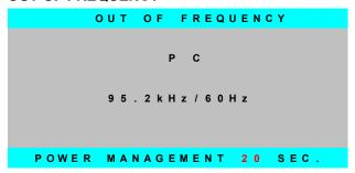
This is when Input Signal is over the range or frequency.
