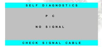
This is when Input Signal is not present after power on with power switch.
