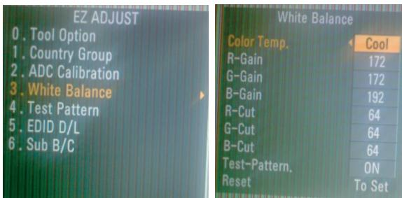
\* After done all adjustments, Press "In-start" button and compare Tool option and Area option value with its BOM, if it is correctly same then unplug the AC cable. If it is not same, then correct it same with BOM and unplug AC cable.
