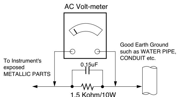
When 25A is impressed between Earth and 2nd Ground for 1 second, Resistance must be less than  $0.1 \Omega$
