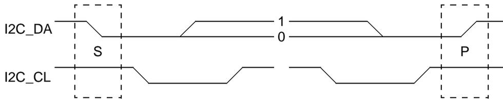
**Fig. 3–1:** I<sup>2</sup>C bus protocol (MSB first; data must be stable while clock is high)
