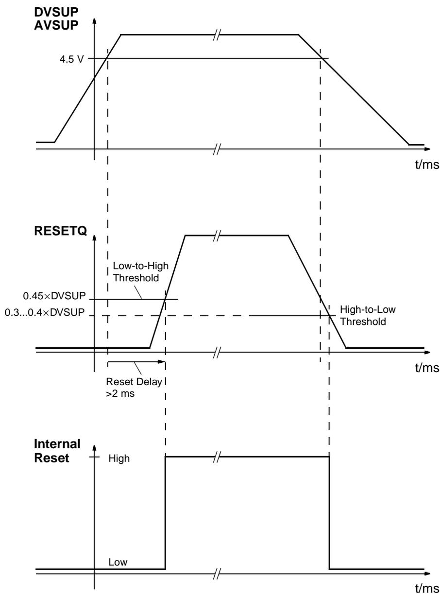
**Note:** The reset should not reach high level before the oscillator has started. This requires a reset delay of  $> 2 \text{ ms}$
