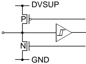
Fig. 4-19: Input/Output Pins: I2S\_CL, I2S\_WS, D\_CTR\_I/O\_1, D\_CTR\_I/O\_0
