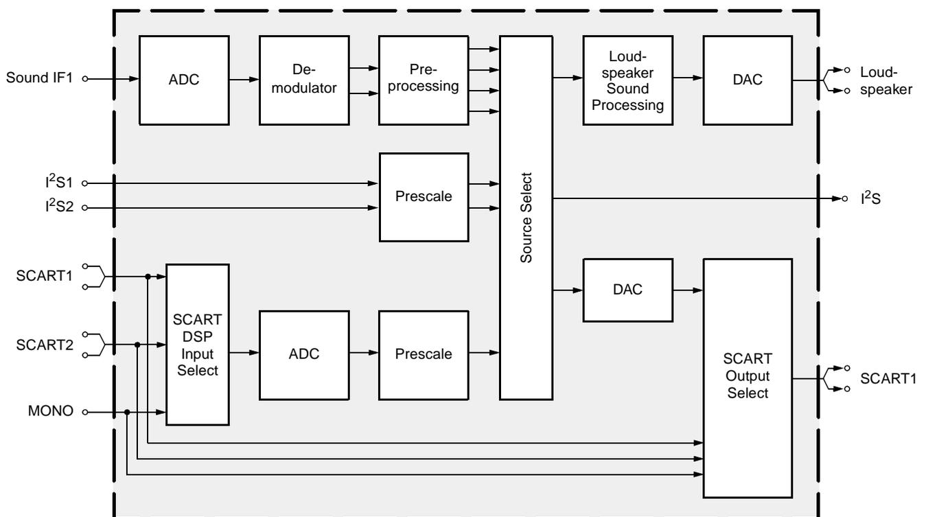
**Fig. 1–1:** Simplified functional block diagram of MSP 34x5G
