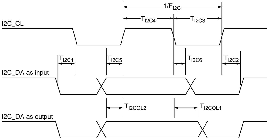
Fig. 4–27: I<sup>2</sup>C bus timing diagram
