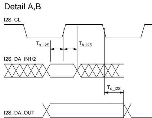
Fig. 4–28: I<sup>2</sup>S timing diagram
