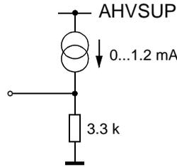
Fig. 4-21: Output Pins: DACM\_R/L
