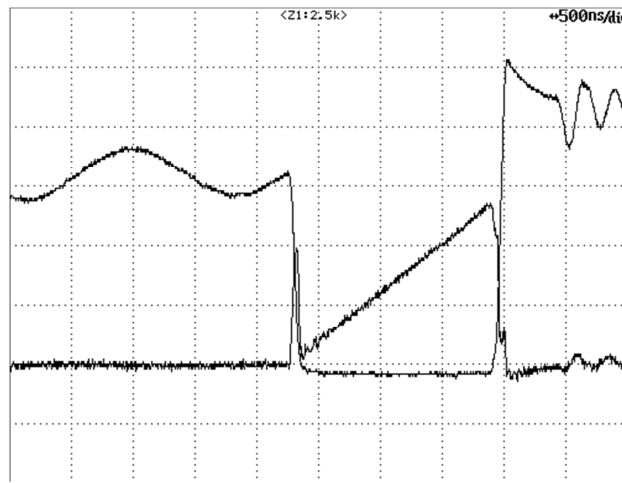
Figure 13 – 230 VAC, Full Load. Upper: I_{DRAIN} , 0.1 A / div. Lower: V_{DRAIN} , 100 V / div.
