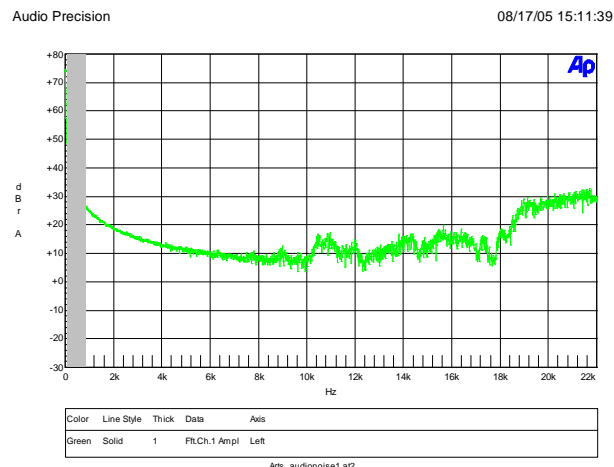
Figure 30 – Audible Noise V_{IN} = 120 VAC; I_{OUT} = 1 A.
