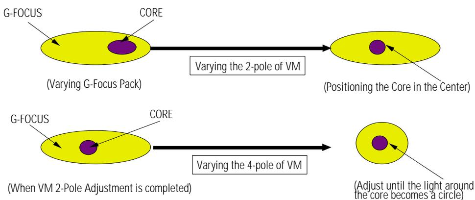
3. Adjust the G-Focus until any light around the core disappears.
