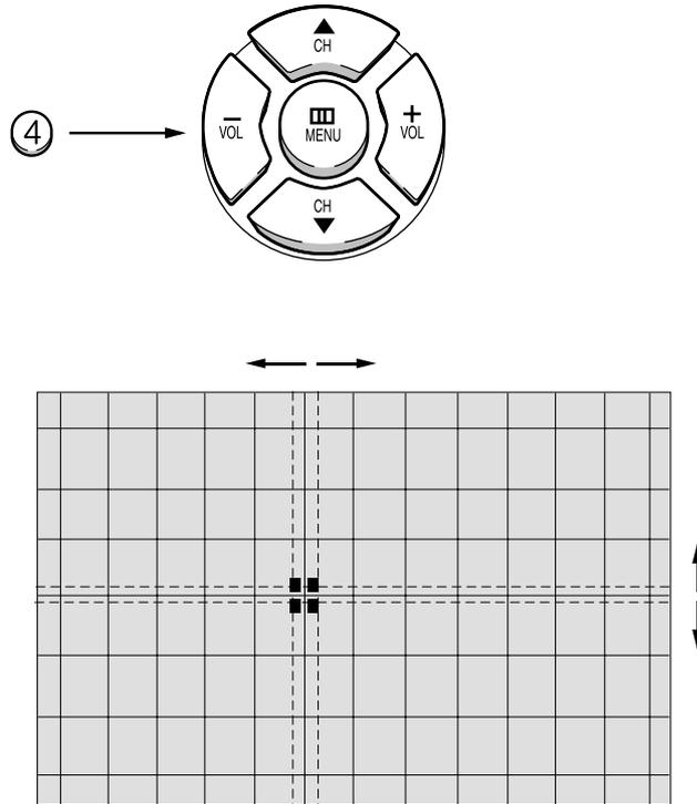
8. After the Line Shift is cancelled by pressing the
