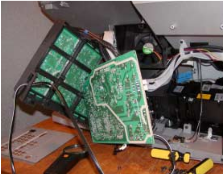
POWER INPUT BOARD IN SERVICE POSITION
