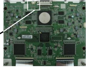
Check for 12V Voltage supplied from P803 Pins 1-2 and/or P802 pins 49-51.
