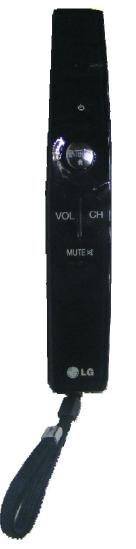
The first time the Motion Remote has it's batteries installed and pointed at the Television, the Motion Remote is synchronized with the TV. After that, when pointing the remote at the TV and pressing the Enter key, a pointer appears on screen, then by moving the Motion Remote around, the pointer moves with the movement of the remote. When the pointer is placed over a selectable button, you can press the center "Enter" button and active the object. This makes navigation much easier.
