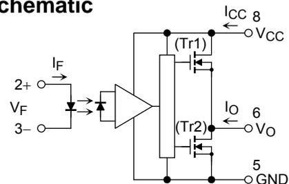
A 0.1  $\mu F$  bypass capacitor must be connected between pins 8 and 5. (See Note 6)
