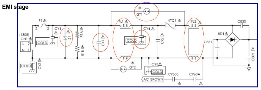
Key components for EMI solution: CX1& CX2 FL1 & FL2
