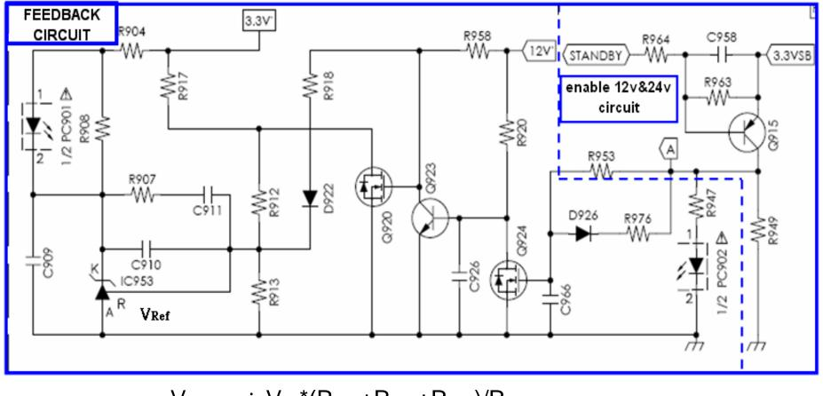
$$V_{out_{3.3V}} = V_{ref} (R_{917} + R_{912} + R_{913})/R_{913}$$
