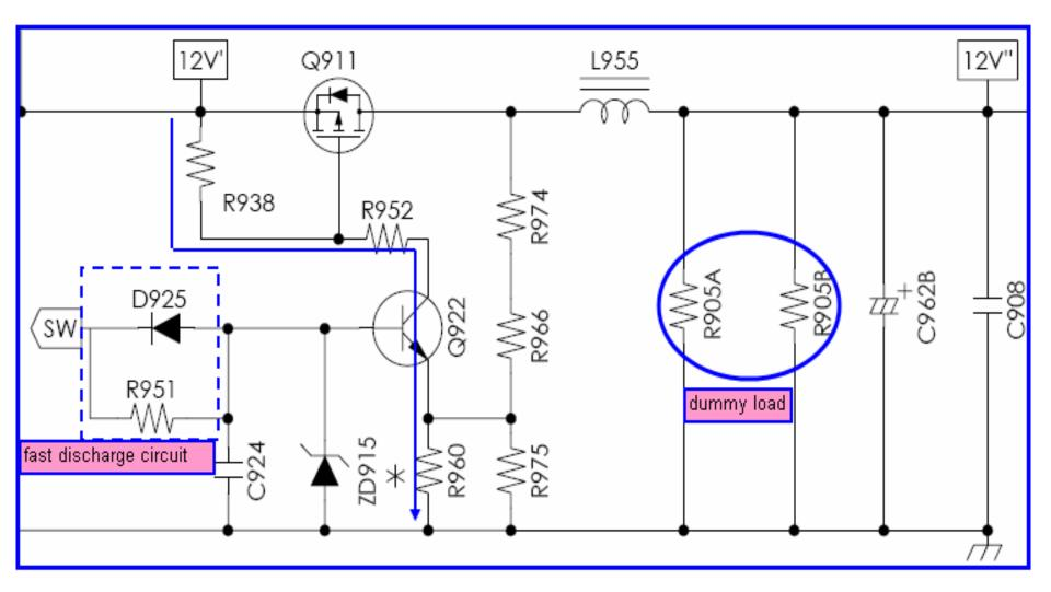
Q911 will be off under standby mode, so that the power saving performance would be better because there's no power loss on R905A/B. R905A/B are used to stabilize the output @ light load condition.
