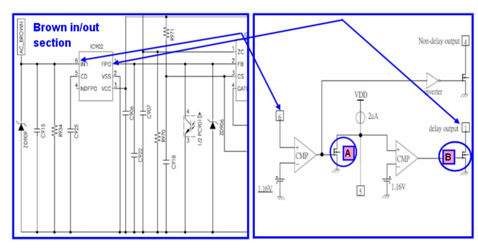
• Notes: IC902 is used to set the AC Brown In/Out point and discharge time. The trigger point is 1.28v for Brown/In and 1.16V for Brown out.
