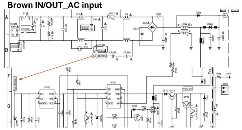
Note: C963A/C963B/R934/IC902 are used to set Brown in/out point. The PSU will be Disabled if IC902 pin6<1.16V, and enabled if IC902 pin6>1.28V.
