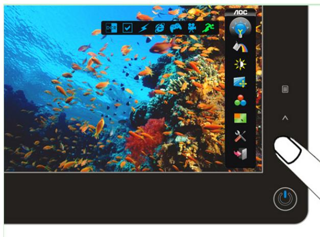
Notes : When Eco mode is not set as “Standard”, Contrast and Brightness can not be adjusted; When DCR is set as “On”, Contrast, Brightness, Eco mode and Gamma can not be adjusted.
