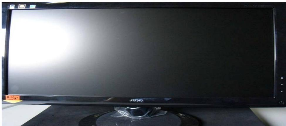
2.Lay down the monitor, then use cross screwdriver or the expert tools leave off the stand while press the Push area of the back cover.
