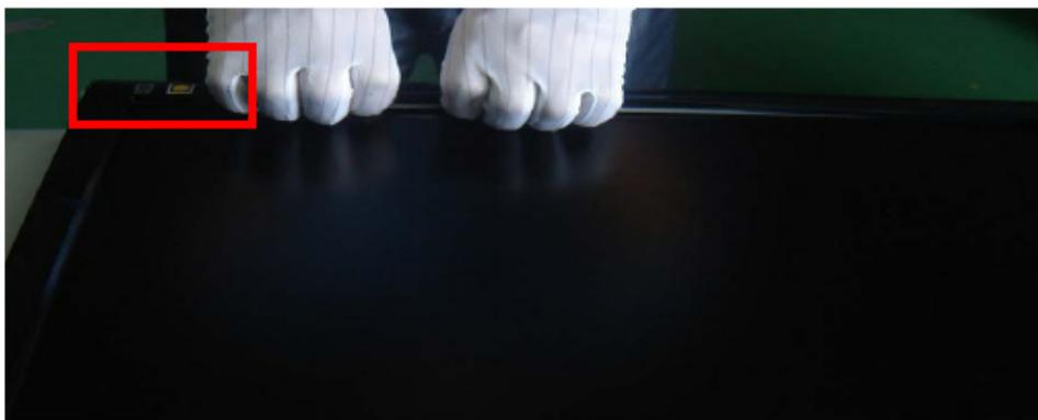
5. As the center of one side of USB connector, take apart 3 sides and stop. Attention: Do not break off the key pc side, or pull the front frame forcibly, to avoid the keypad peel off.
