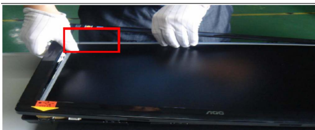
6. Overturn the monitor, on the USB connector area, one hand press the Panel, and use the other to undraw the back cover.
