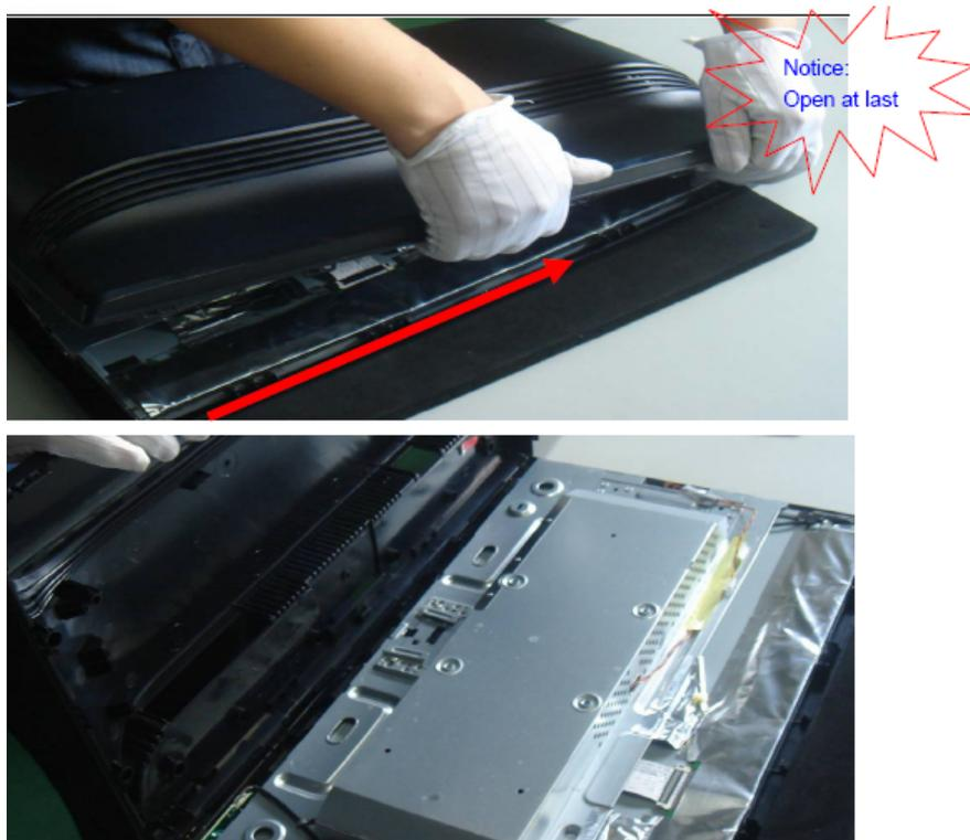
8. In turn to take apart the key pc connect PIN (A&B), lamp line (C&D), peel off the aluminum foil (E&F), draw off the FFC pin (G), if there is defect with main pc, need leave of f the six-angle screw (H).
