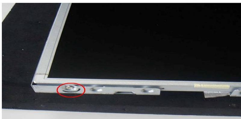
10. According to the different defective area, take off the screws ABCDE to get the relevant part to maintain. Before take apart the POWER pc should take off the AC iron piece first.
