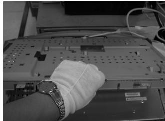
6. Disconnect cable and lift up the main board and panel shield. (see illustrations)
