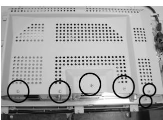
4. Remove 2 screws (A/V Input Board) from the shield. Please add a circle around the 6 screws that connects the silver shield of the Main-PCB to the Panel shield.(see illustrations)
