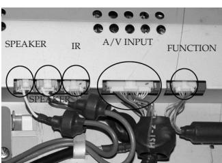
3. Lift up the rear cover and disconnect function cable, A/V Input cable, IR cable and speaker cable from the shield. (See illustrations)
