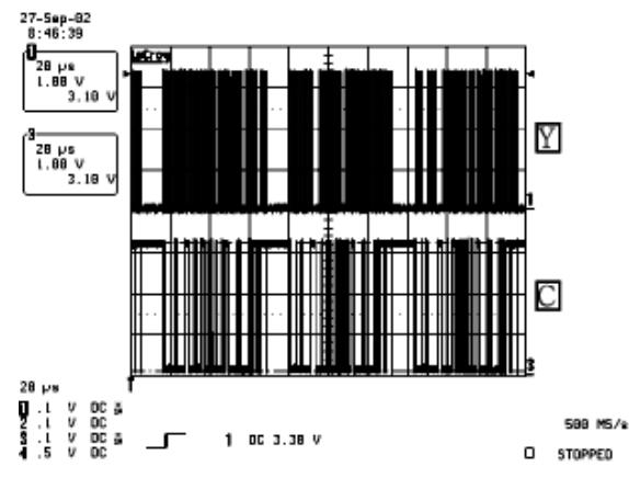
**11** Digital Output Y,C\_OUT (0:7) Data Of IC405
