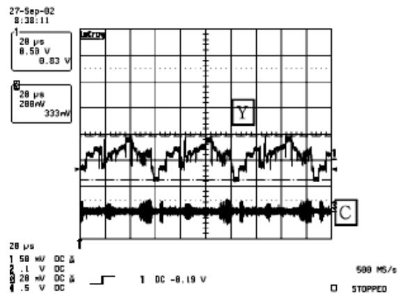
**10** 3230 Y,C\_OUT (0:7) Data
