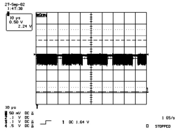
**9** Analog Signal (Y,C) to IC201
