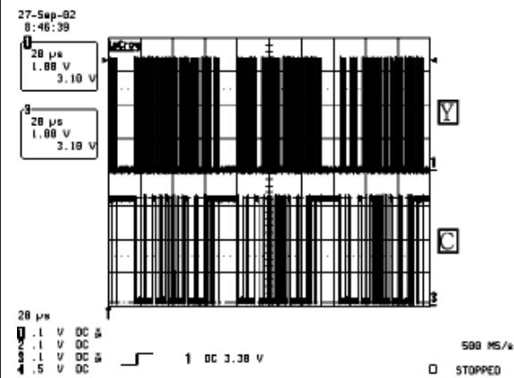
**11** Digital Output Y,C\_OUT (0:7) Data Of IC405
