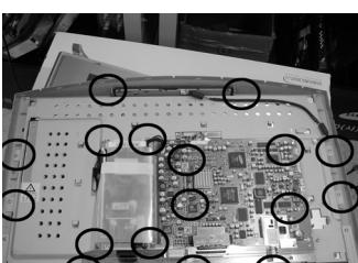
5. Lift up main shield and remove 17 screws from the set (Main Board and Panel Shield). (see illustrations)
