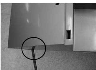
2. Remove 2 screws from the rear cover and remove rear cover by using opening driver.
