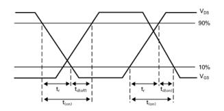
Switching time waveforms
