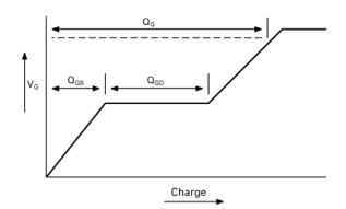
Basic gate charge waveform
