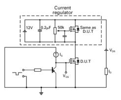
Gate charge test circuit
