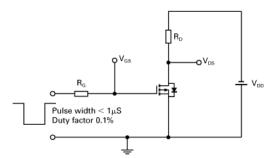
Switching time test circuit
