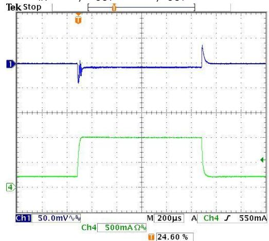
$V_{IN} = 5V, V_{OUT} = 3.3V, I_{OUT} = 0.2A \leftrightarrow 1A$
