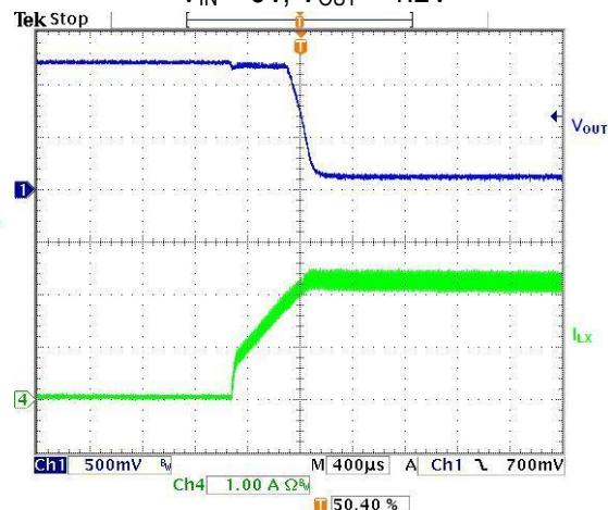
$V_{IN} = 5V, V_{OUT} = 1.2V, I_{OUT} = 0.2A \leftrightarrow 1A$
