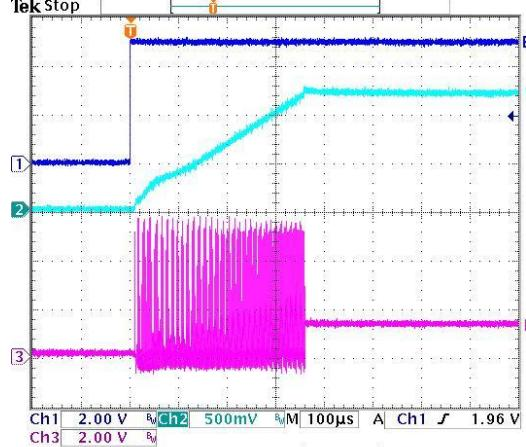
$V_{IN} = 5V, V_{OUT} = 1.2V, R_{LOAD} = 1\Omega$
