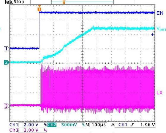
$V_{IN} = 5V, V_{OUT} = 1.2V, R_{LOAD} = \text{No Load}$
