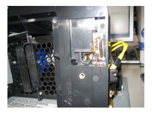
6. Disconnect the ballast cable and remove the ballast unit from the retaining clips 1 - 4.
