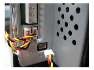
2. Remove the DMD Fan casing by removing screws 1, 2, and 3.
