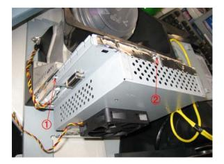
5. Remove the DMD Fan by removing screws 1 and 2.
