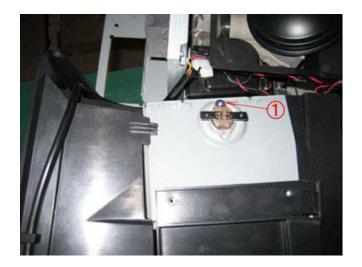
(Thermostat Breaker is secured by 2 screws in some production units.)
