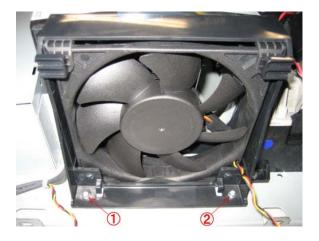
4. Remove the 4 rubber corners from the old lamp fan and place them on the new lamp fan.
