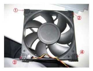
5. Assemble the new fan to the light engine by following steps 1-4 in reverse.
