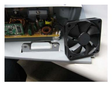
3. Fix the Ballast Fan with two pins.
