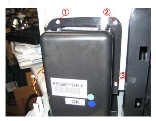
3. Remove the 2 screws securing the LVDS connector.
