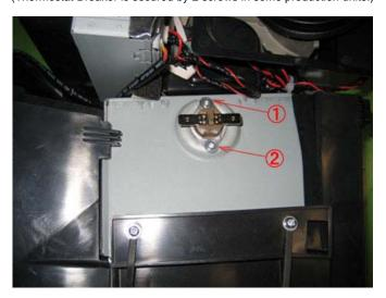
3. Reconnect the thermostat lead wires.
