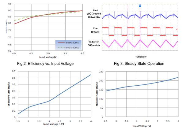
Fig 4. Shutdown Current vs. Input Voltage
