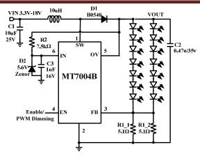
Fig 13. Driving 14 WLEDs (7WLEDs in Series and 2Strings Paralleled) with 3.3V-18V Input Voltage
