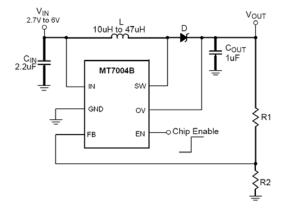
Fig.19 Constant output voltage application
