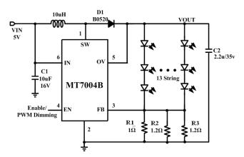
Fig 11. Circuit for Driving 39 WLEDs (3 WLEDs in Series and 13 Strings Paralleled)
