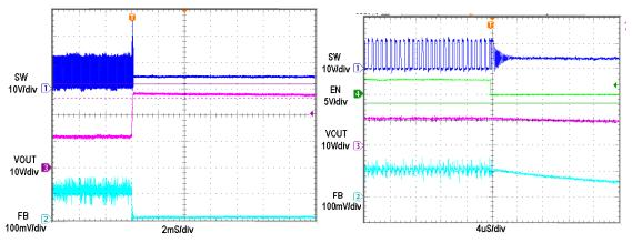
Fig 8. Open Load protection
