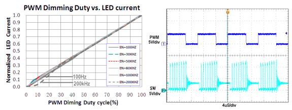
Fig 6. EN PWM dimming vs. LED Current
