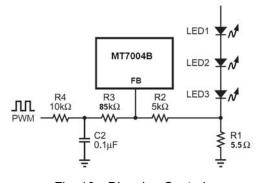
Fig. 16 Dimming Control Using a Filtered PWM Signal
