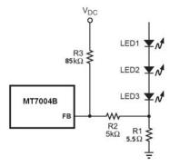
Fig. 15 Dimming Control Using a DC Voltage
