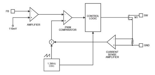
Fig 1—Functional Block Diagram
