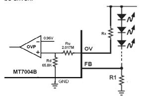
Fig. 18 OVP topology with external resistor
