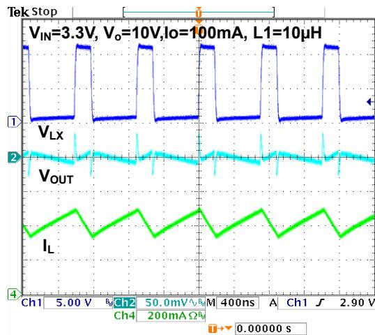
Figure 18. Operation Waveform
