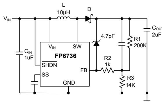
Figure 22. With Open-Circuit Protection
