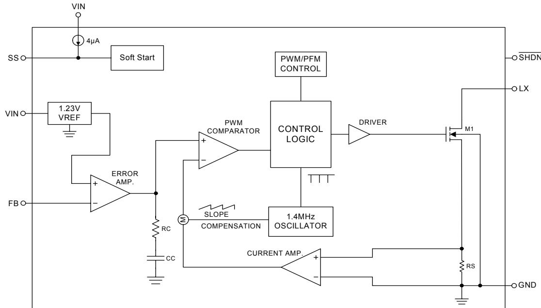
Figure 5. Block Diagram of FP6736
