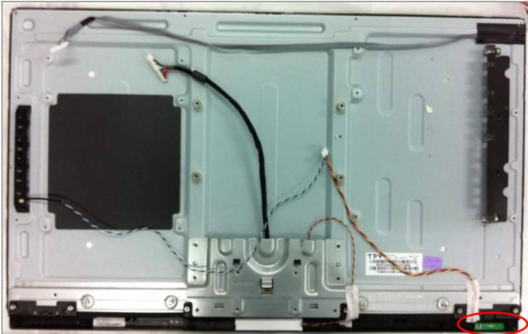
5. Remove the screws to remove the Panel.
