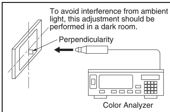
**Note:** The optical receptor must be set perpendicularly to the LCD Panel surface.
