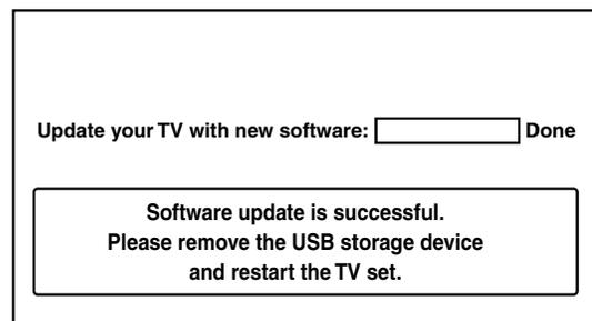
Remove the USB storage device from the USB port. Turn the power off and turn the power on again.
