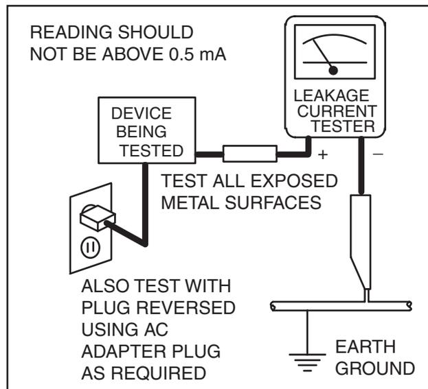
**ANY MEASUREMENTS NOT WITHIN THE LIMITS SPECIFIED HEREIN INDICATE A POTENTIAL SHOCK HAZARD THAT MUST BE ELIMINATED BEFORE RETURNING THE INSTRUMENT TO THE CUSTOMER OR BEFORE CONNECTING THE ANTENNA OR ACCESSORIES.**
