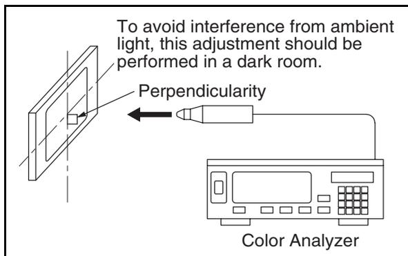
**Note:** The optical receptor must be set perpendicularly to the LCD Panel surface.
