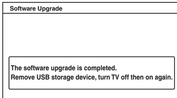
Remove the USB storage device from the USB port.
