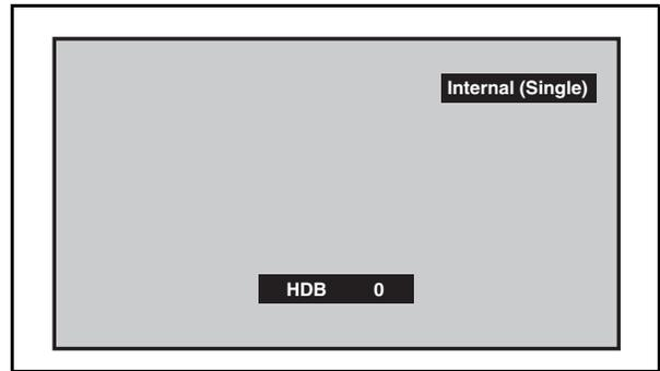
7. Press [CHANNEL UP/DOWN] buttons to adjust the color temperature becomes  $12000^{\circ}\text{K}$  ( $x = 0.272 / y = 0.278 \pm 0.003$ ).
