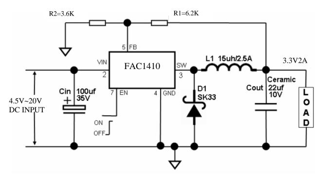
Fig11. Typical Application Circuit (with ceramic output capacitor) @ 3.3V/2A
