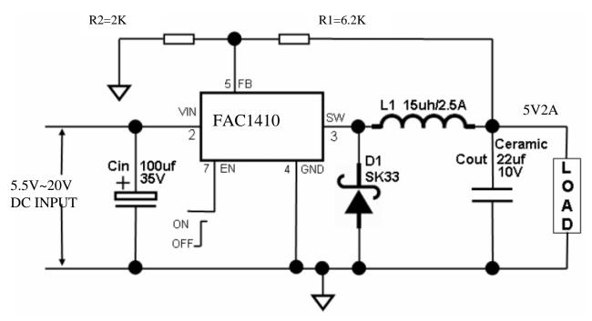
Fig10. Typical Application Circuit (with ceramic output capacitor) @ 5V/2A
