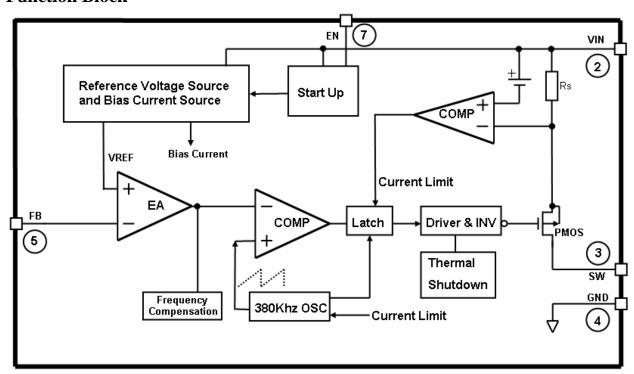
Figure 3 Function Block Diagram of FAC1410
