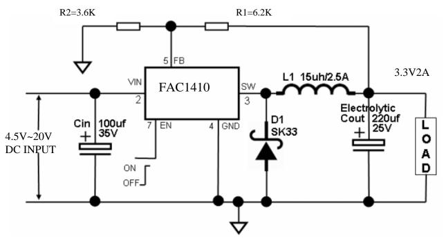
Fig9. Typical Application Circuit @ 3.3V/2A
