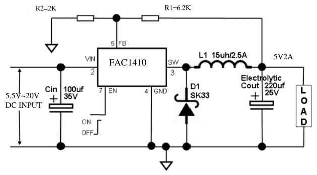
Fig8. Typical Application Circuit @ 5V/2A
