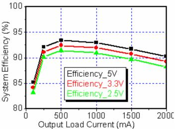
Figure 7. Efficiency vs. Load (Vin=10V)
