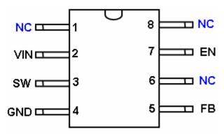
Figure 2 Pin Configuration of FAC1410 (Top View)
