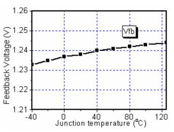
Figure 5. Vfb vs. Temperature
