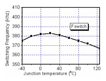
Figure 4. Switching Frequency vs. Temperature
