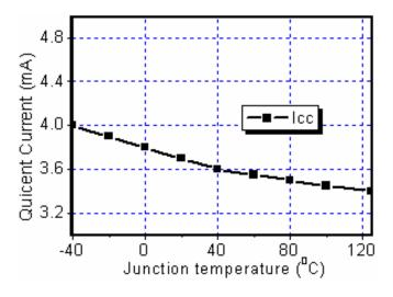
Figure 6. Icc vs. Temperature
