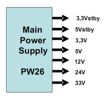
17MB70 general power managment block diagram is shown below. 17PW26 power board is used in 32" 17MB70 TV sets.
