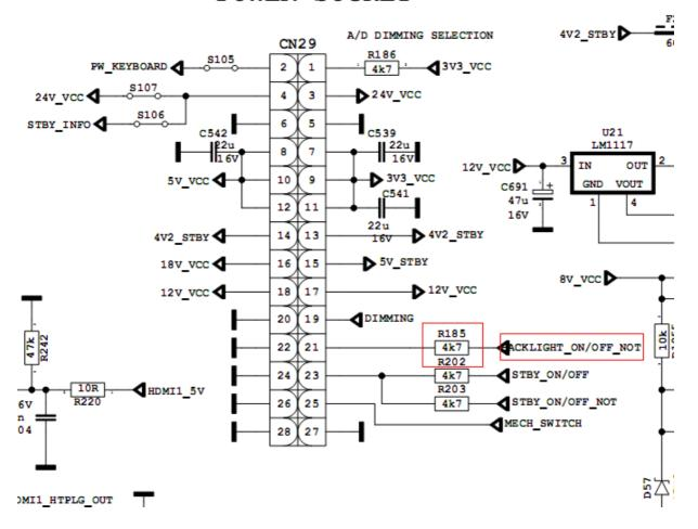
Dimming pin should be high or square wave in open position. If it is low, please check S32 for BRCM side and panel or power cables, connectors.
