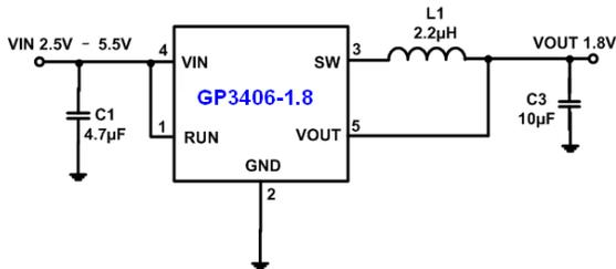
Figure 4. Basic Application Circuit with fixed output versions
