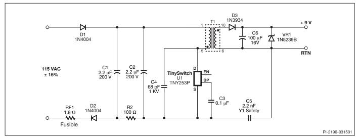
Figure 12. 0.5 W Open Loop AC Adapter Circuit.
