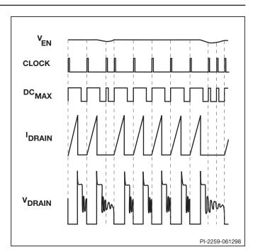
Figure 5. TinySwitch Operation at Medium Load.
