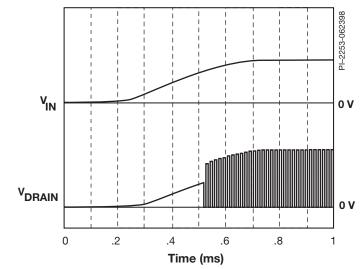
Figure 7. TinySwitch Power-Up Timing Diagram.
