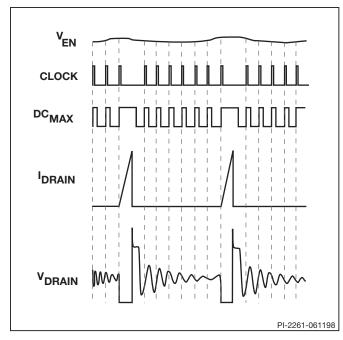
Figure 6. TinySwitch Operation at Light Load.
