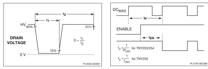
Figure 15. TinySwitch Duty Cycle Measurement.
