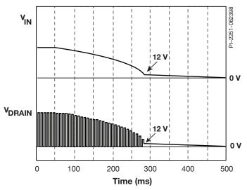
Figure 8. TinySwitch Power Down Timing Diagram.
