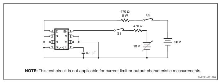
Figure 14. TinySwitch General Test Circuit.
