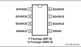
Figure 3. Pin Configuration.
