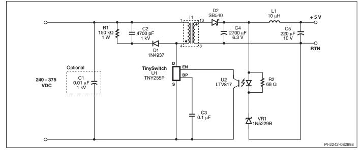
Figure 10. 10 W Standby Supply Circuit.
