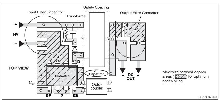
Figure 13. Recommended PC Layout for the TinySwitch.
