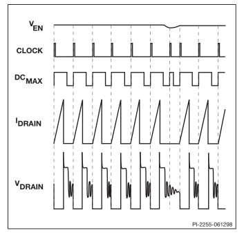
Figure 4. TinySwitch Operation at Heavy Load.
