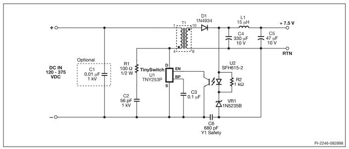
Figure 9. 1.3 W TV Standby Circuit using TNY253.
