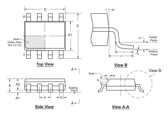
**Note 1:**This chamfer feature is optional. If it is not present, then a Pin 1 identifier must be located in the index area indicated. The Pin 1 identifier may be either a mold, or an embedded metal or marked feature.
