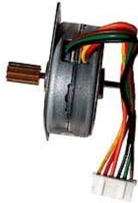
This stepper motor costs less than \$2.00 from [BG Micro](#) and has 6 wires as shown in the diagram above.
