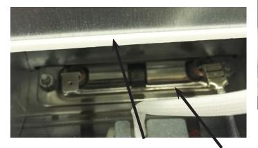
At the front of the broil element is a broil guard mounted with two screws. Remove the guard (the front of the element will drop down a few inches).
