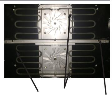
After you remove the convection cover from the back of the oven, You can see that the heating element and fan blades are accessable. Remove 4 screws from around the silver panel and pull the heating element and silver panel out toward you. The assembly will not move to far until you disconnect the 6 electrical connections. One quick disconnect plug from each motor and 2 spade terminal connections for the heating element. Once these are removed the assembly can be removed grom the oven.
