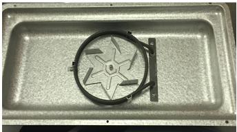
With the mounting panel removed, turn the panel over to view the Convection Fan and Convection burner element.
