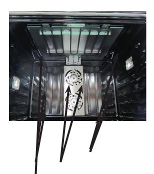
From inside the oven, remove 8-10 mounting screws around the Convection cover.
