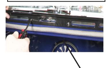
Open the oven door to expose the vent trim located above the oven door opening.
