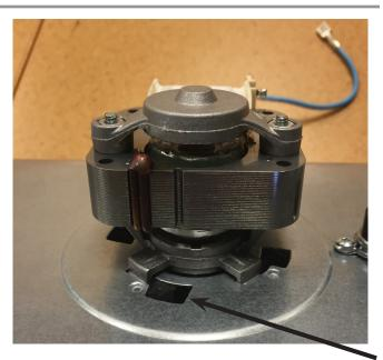
To remove the Fan Motor, you need to remove the Fan Blade (the fan blade has a "D" shaft cutout on the fan blade for easy re-assembly).
