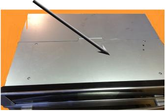
With the Top Control Service Cover removed, the Microwave service compartment panel is exposed. Remove the mounting screws from the panel. Lift the front of the panel and slide the panel toward the front of the oven and remove it.
