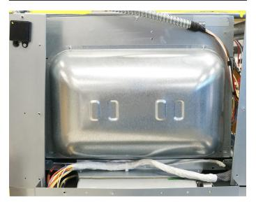
All components are accessed from the back of the oven. To gain access to the Microwave Convection parts, the Oven will need to be removed from the installation.
