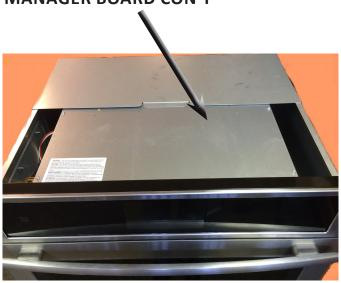
After sliding the cover panel out, access to the Microwave Oven Appliance Manager board is available. Remove the Appliance Manager mounting screws and electrical connections and remove the board.
