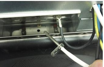
Below, from inside the oven cavity. The Broil element is shown at the top of the cavity and the Humidity sensor is shown at the back of the oven suspended from the ceiling.
