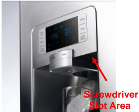
Insert a flat-blade screwdriver into slotted area as shown in photo right. After inserting the screwdriver into the slotted area, place one hand underneath the panel, while twisting the screw driver CCW pull the panel out toward the front until the right side pops out. Once the right side pops out the panel is easily removed.
