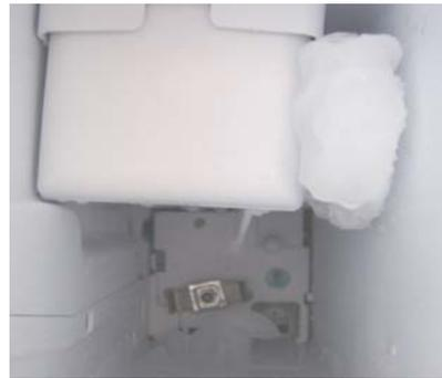
**CAUSE: When the ice tray dumps ice cubes to the ice bucket, ice cubes jam between the ice tray and the liner. The ice maker makes a loud noise and eventually stops working.**
