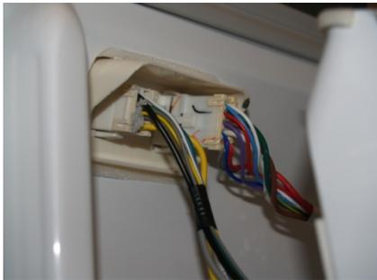
Auger/ice maker ass'y has plastic that locks into the two pieces on the door liner
