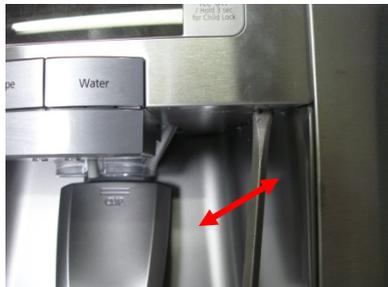
**DO NOT** try and pry the panel out by pushing, or pulling the screwdriver. This will only damage the slotted area.
