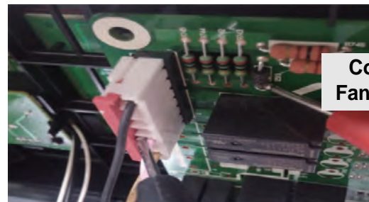
1st pin of CN62 and cathode of D503 : RY 61
