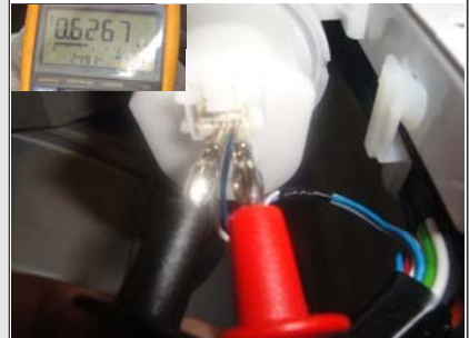
PICTURE E7-3: Water level sensor is being checked.
