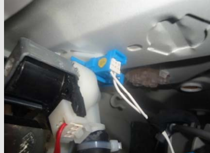
Picture E15-2: Is the flowmeter socket on the water inlet valve fitted?
