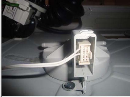
Picture E12-1: Aquastop connections at the lower section of machine
