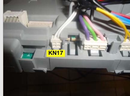
Picture E12-2: KN17 socket Aquastop (White-White) connections
