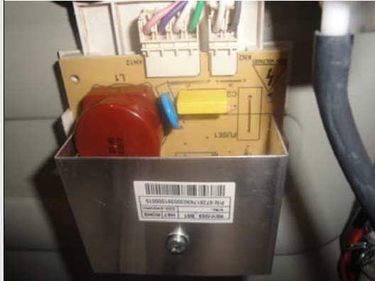
PICTURE-5 MOTOR DC CARD sockets KN2- UMDC MOTOR KN12- THERMOCOUPLE KN12- UMDC MOTOR WINDING
