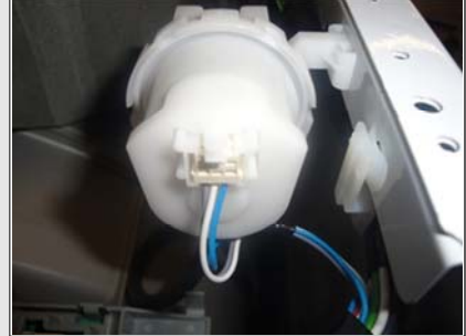
PICTURE E7-1: Socket on the level sensor should be fitted.
