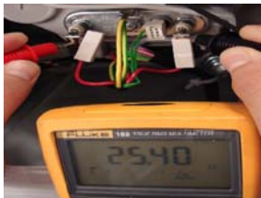
PICTURE E3-3: One of the cables on the heater is removed (left) and heater resistance is measured.
