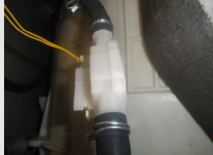
Picture E15-3: Is the flowmeter socket on the water inlet hose fitted?
