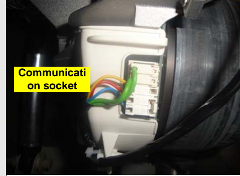
Picture E13-2: Communication connector connection on the motor
