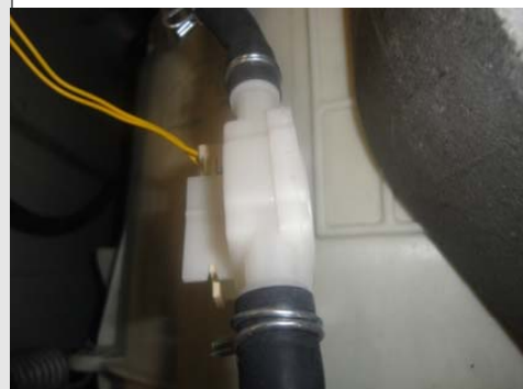
Picture-1_1 : Flowmeter CORRECT assembly
