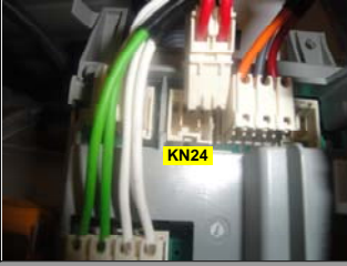
PICTURE E3-1: Heater socket on the KN24 card was removed.
