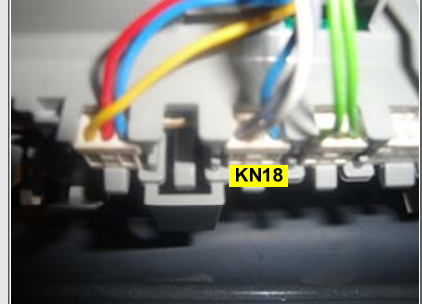
PICTURE E7-2: Socket to which the KN18 level sensor cables are fitted
