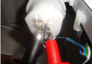
PICTURE E3-4: Water level sensor is being checked.
