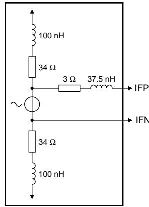
Fig 7. Typical IF output impedance at 10 MHz
