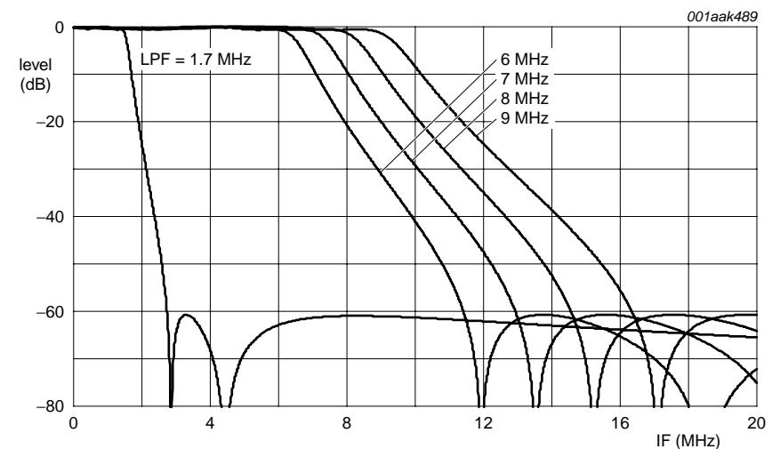
Fig 10. Low-pass filter
