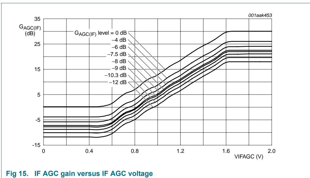
Fig 15. IF AGC gain versus IF AGC voltage
