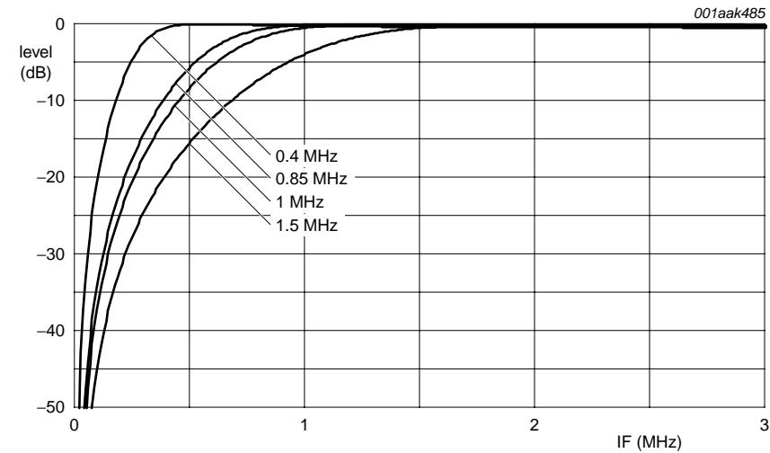
Fig 11. High-pass filter
