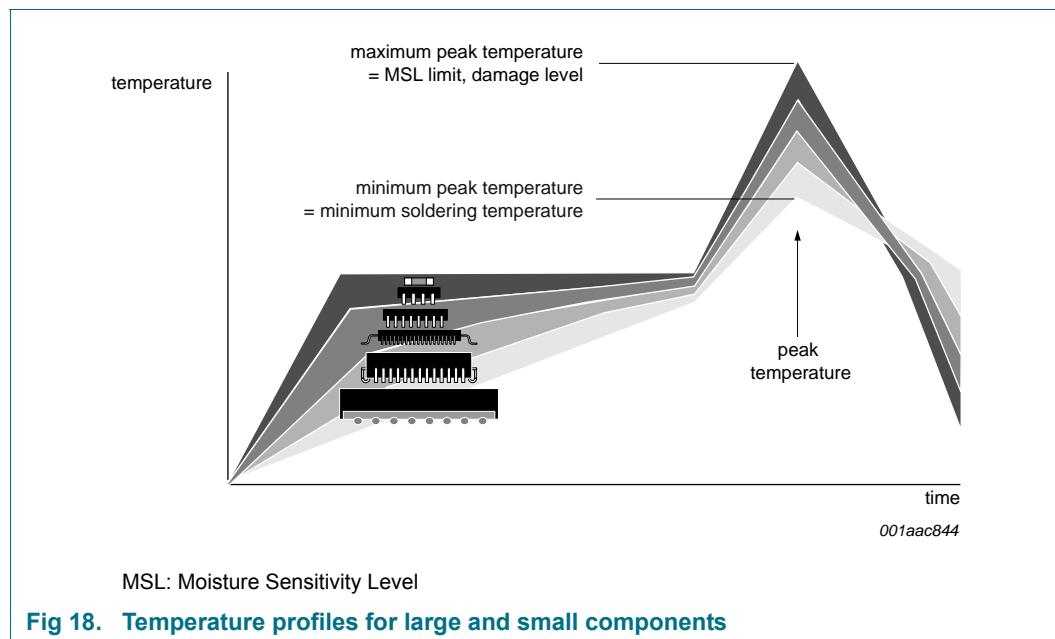
**Fig 18. Temperature profiles for large and small components**
