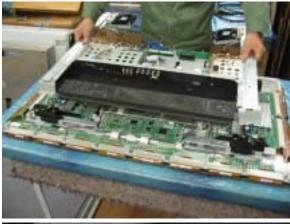
10. Remove the Base Frame together with wires and other parts.
