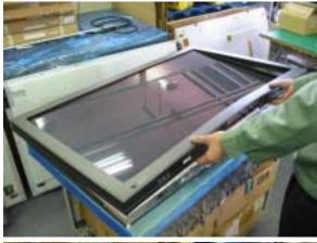
2. Lift the bottom of the Bezel Front.
