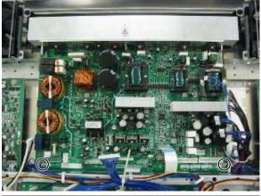
4. Remove the 2 screws and Main Power PCB.
