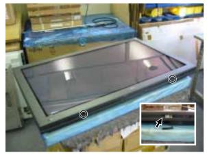
1. Remove the 2 circled Cover Stands and remove the screw in the holes.
