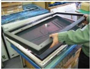
Lift the Bezel Front upward to remove it. (The top of the Bezel Front is hooked.)
