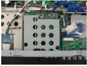
1. Remove the Rear Case and disconnect the circled connectors.
