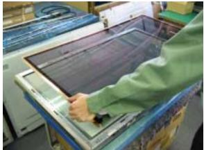
4. Remove the Optical Filter.
