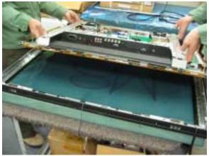
\* View after removal of the Base Frame from the Front Case.
