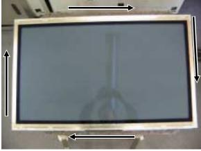
3. Remove by sliding the Filter Holder in the arrow directions.
