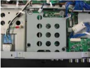
2. Remove the circled 4 screws and the shield bracket.
