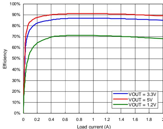
**Efficiency vs. Loading ( $V_{IN} = 5V$ )**
