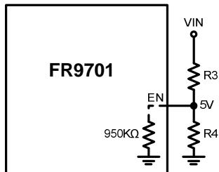
The external resistor divider is used to set the EN automatic startup voltage:
