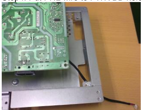
Step5: Connect SPS BD and Speaker By wire
