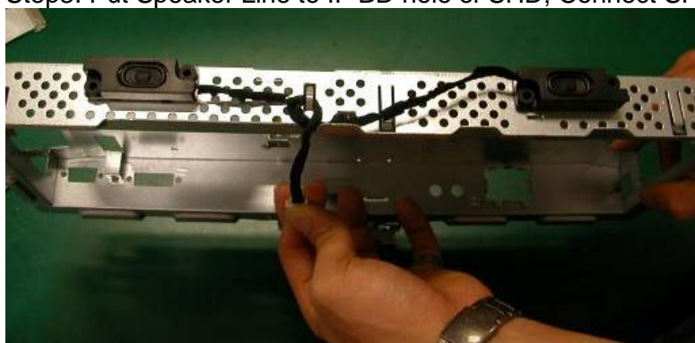
Step4: Put PNL wire to PWR BD hole of SHD:
