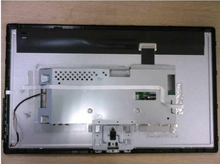
Step10: Put in Tape adhesive to panel wire
