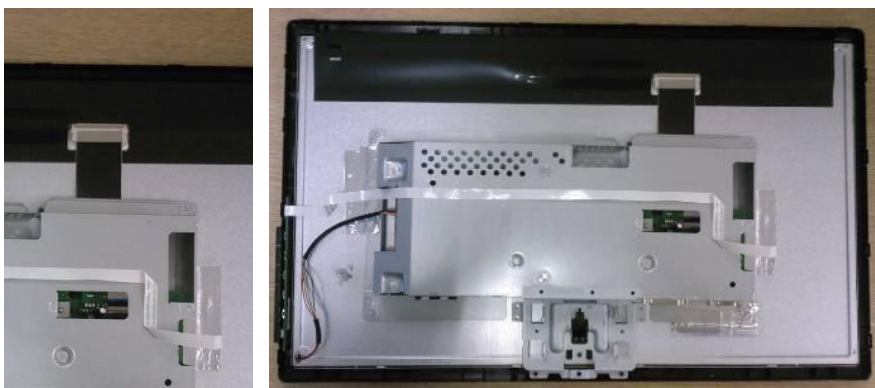
Step7: Put in Tape adhesive to panel wire
