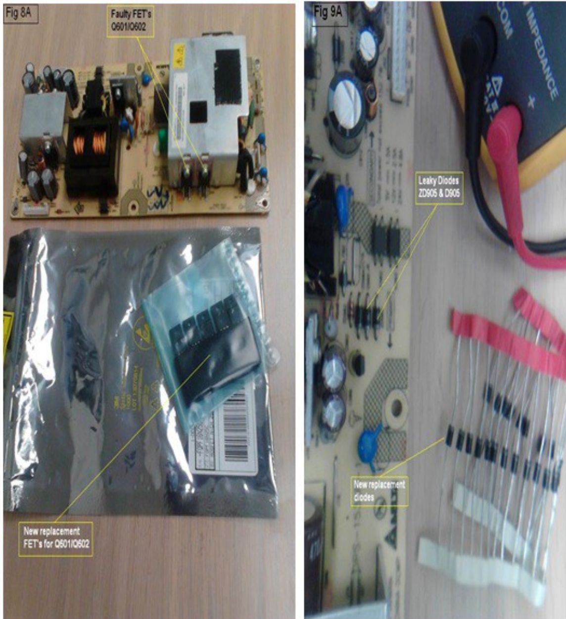
Fig-8A- Identifying faulty MOSFET's and Control IC chip
