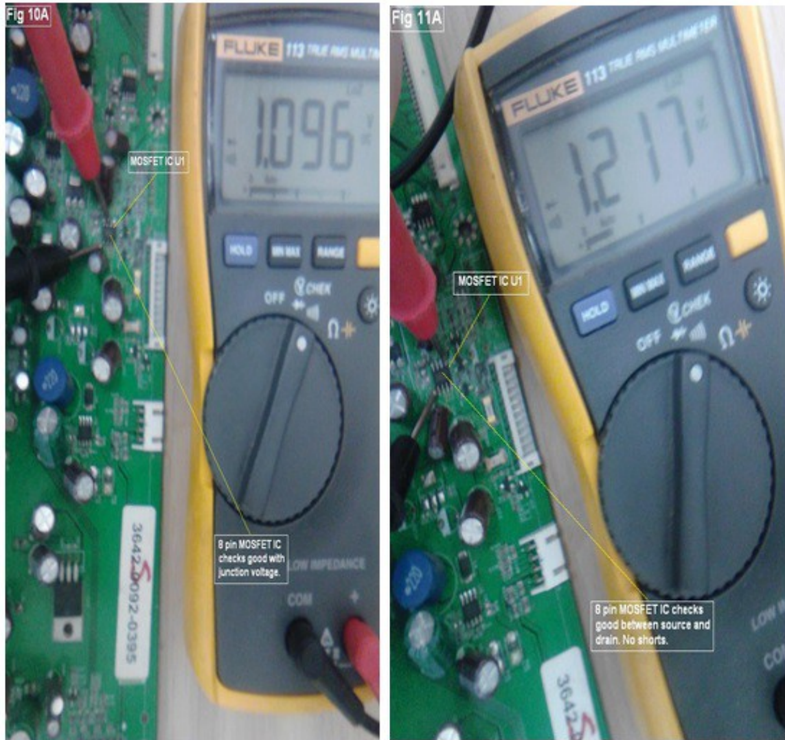
Fig 10A/11A- Vizio main-board part-location number Identifying good MOSFET IC chip
