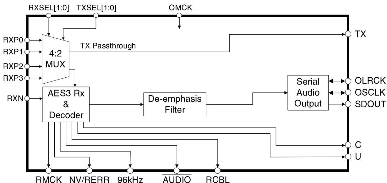
Power supply pins (VA, VD, and VL), AGND, DGND, the reset pin (RST) and the PLL filter pin (FILT) are omitted from the diagram. Please refer to the Typical Connection Diagram for connection details.
