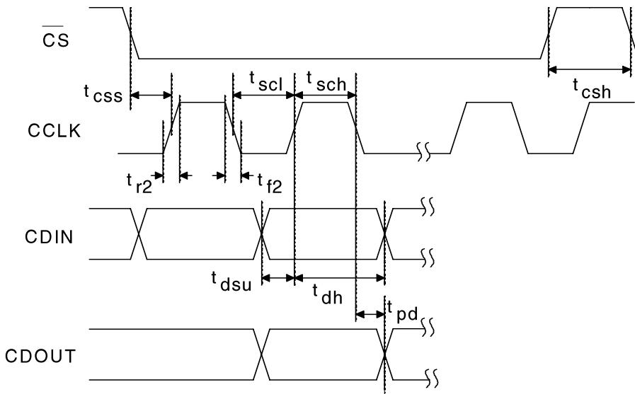
Figure 3. SPI Mode Timing
