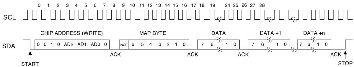
**Figure 12. Control Port Timing, I<sup>2</sup>C Slave Mode Write**
