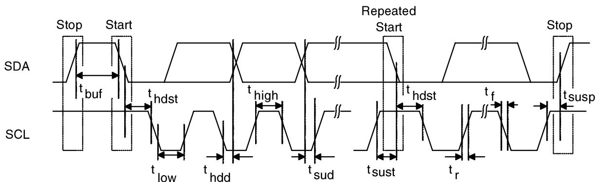
Figure 4. I<sup>2</sup>C Mode Timing
