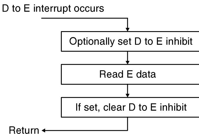
**Figure 22.** Flowchart for Reading the E Buffer
