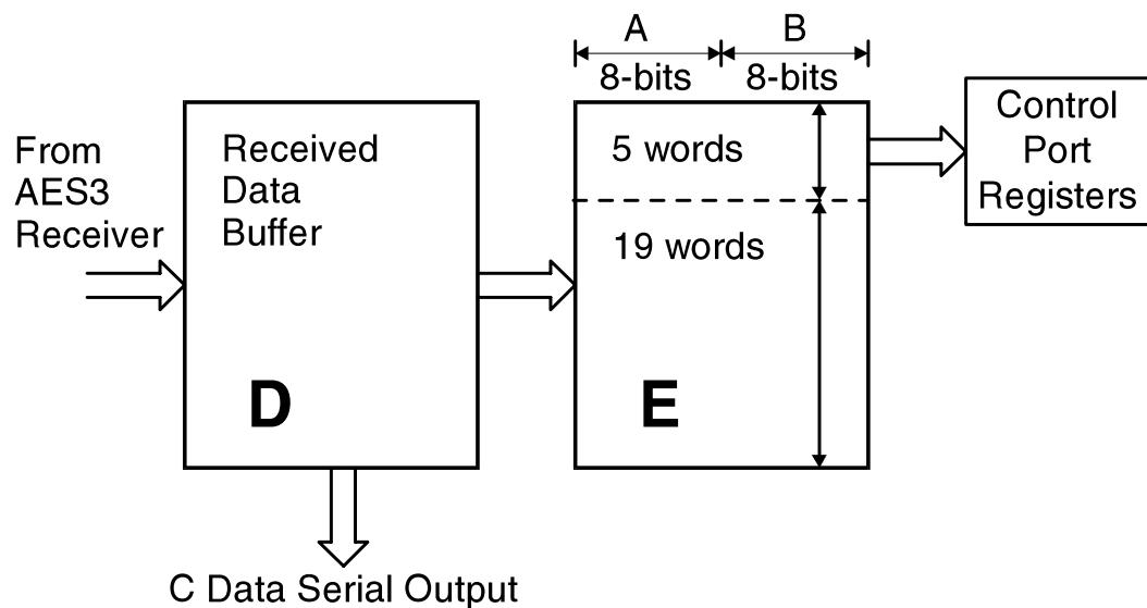
**Figure 21.** Channel Status Data Buffer Structure
