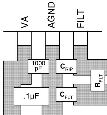
**Figure 24. Recommended Layout Example**
