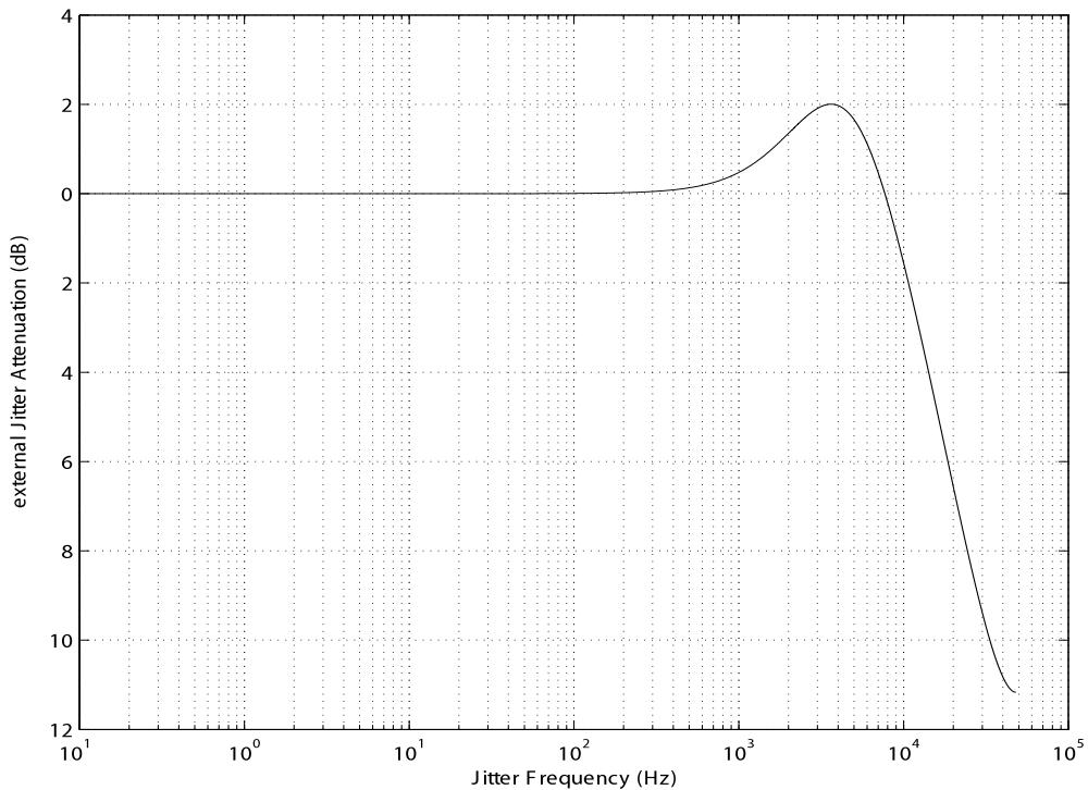
**Figure 25. Jitter Attenuation Characteristics of PLL**
