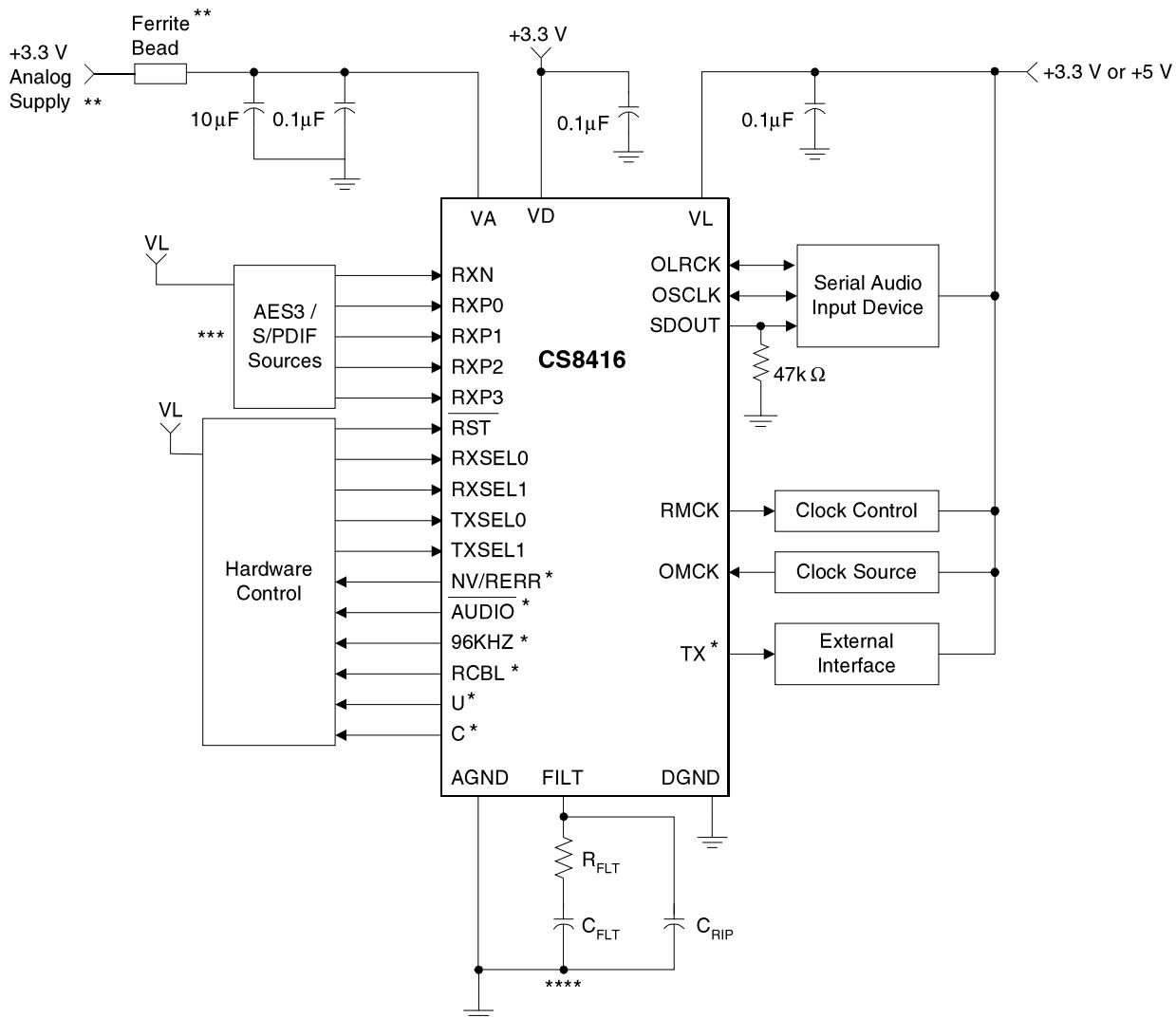
\* These pins must be pulled high to VL or low to DGND through a 47 kΩ resistor.
