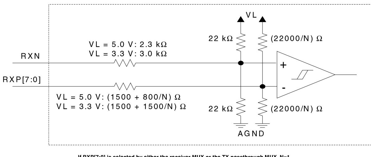
If RXP[7:0] is selected by either the receiver MUX or the TX passthrough MUX, N=1.
