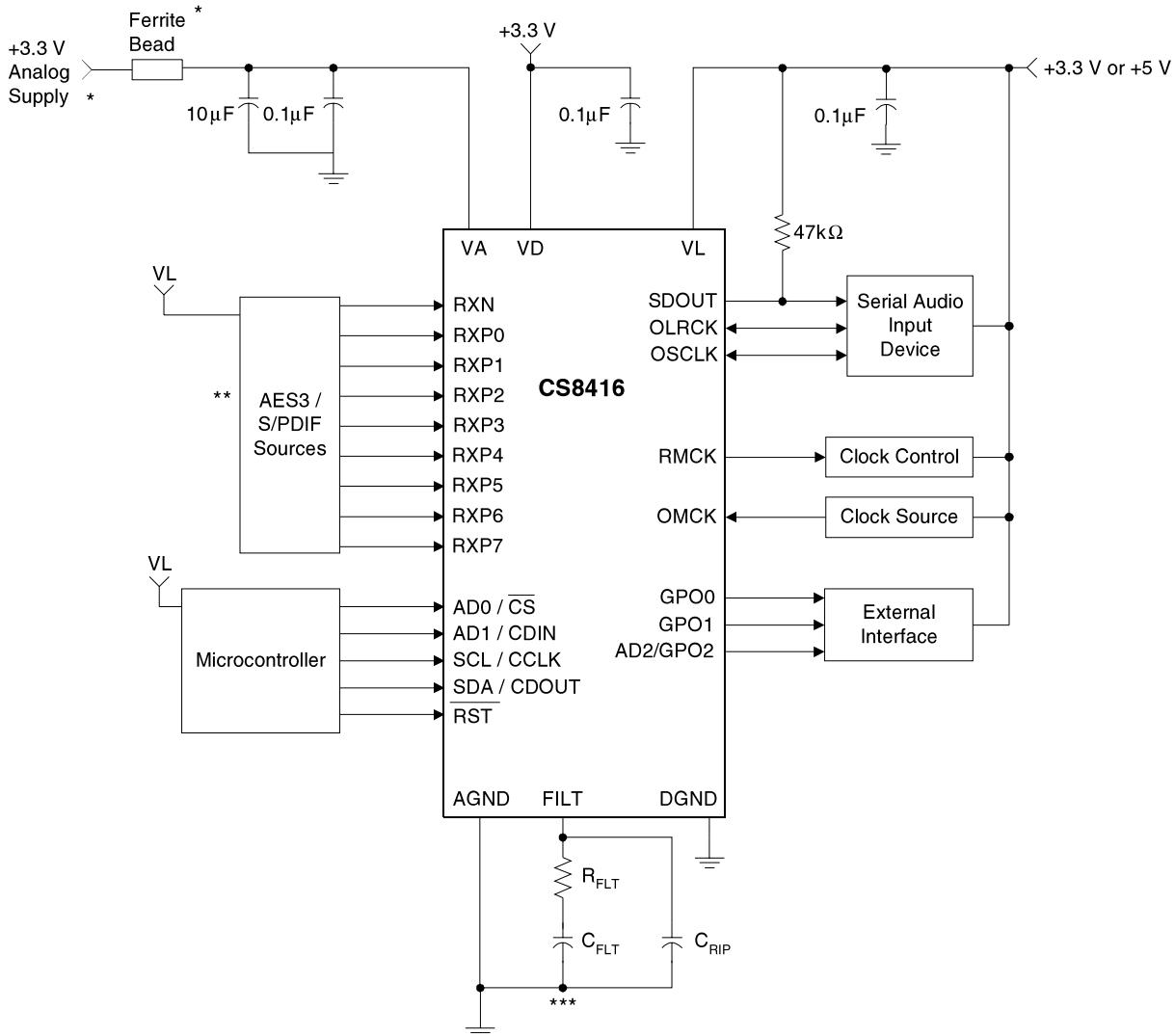
\* A separate analog supply is only necessary in applications where RMCK is used for a jitter sensitive task. For applications where RMCK is not used for a jitter sensitive task, connect VA to VD via a ferrite bead. Keep decoupling capacitors between VA and AGND.
