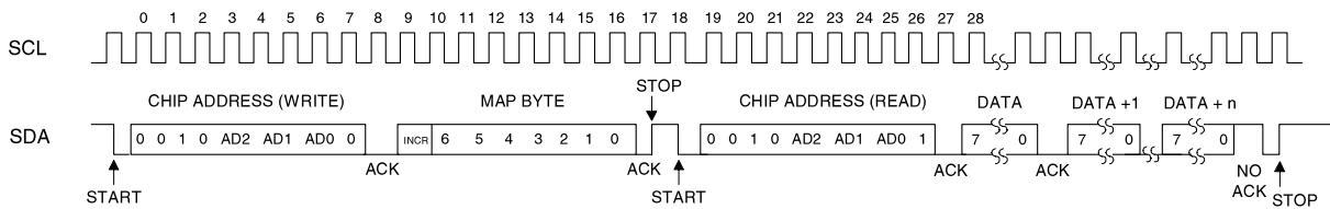
**Figure 13. Control Port Timing, I<sup>2</sup>C Slave Mode Read**
