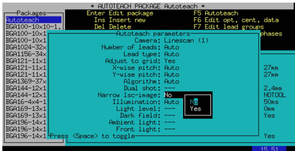
Figure 5: When Autoteaching and picking from feeder the user can now choose between using a narrow or a wide linescan image
