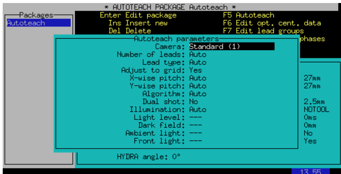
Figure 10. There are now two pitch fields in the window that controls Autoteach of ball devices, one for the x-direction and one for the y-direction
