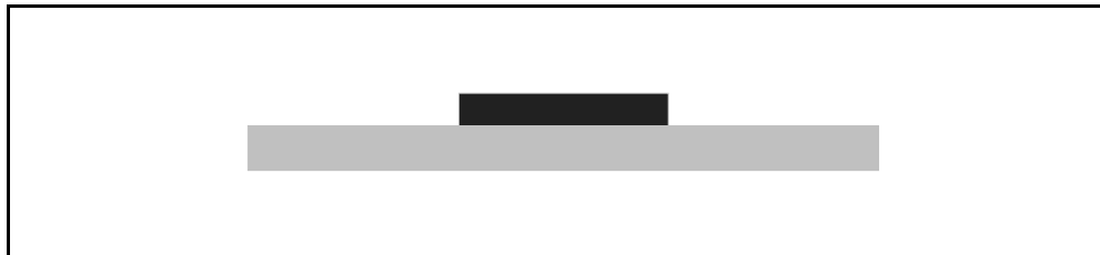
Figure 20. No check is made on overall length or width for mechanical centering. This is done to make it possible to mechanically center components like the one above. The component can be mechanically centered by moving the top part of the component into the centering unit.
