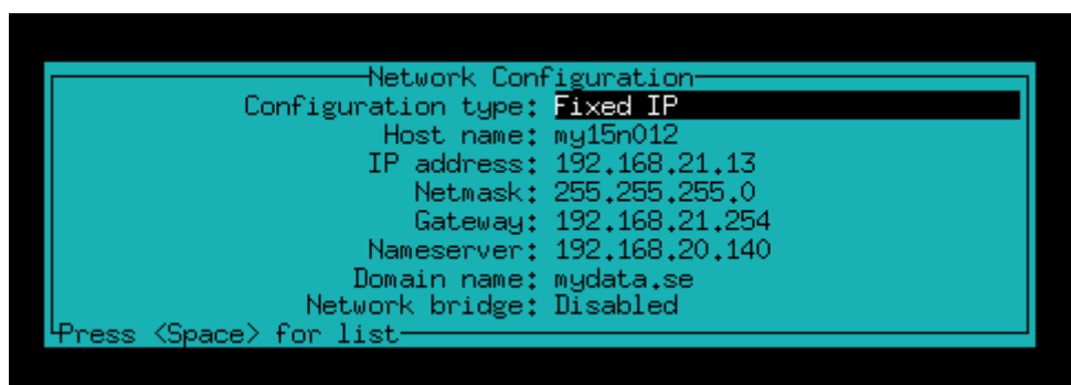
Figure 22. The configuration window in which the network configuration of the machine/server can be set up
