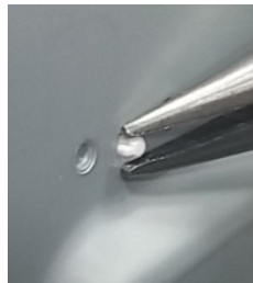
(Step 8) DPS, LED Fixer disassemble & Reflector Sheet disassemble
