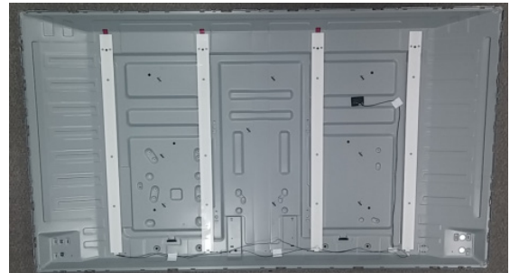
* Finish the Attached Double Tape (3ea)
