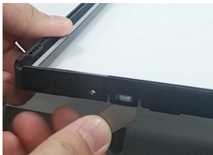
(Step 6) Guide Panel disassemble
