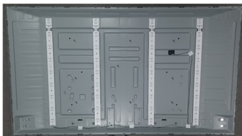
* Finish the Attached LED Array
