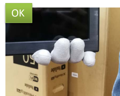
Support set at edge of BZ without touching o-cell
