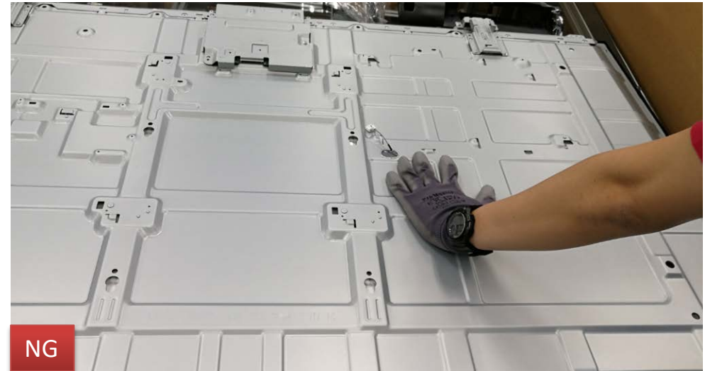
Press on P-mod during assy & disassy
