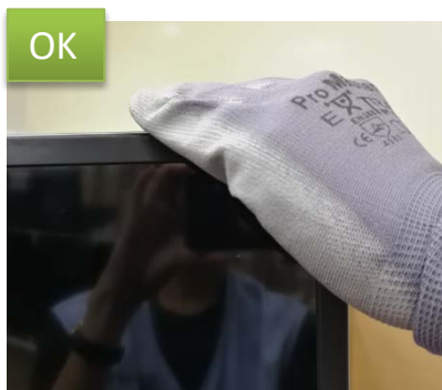
Holding edge of BZ without touching o-cell
