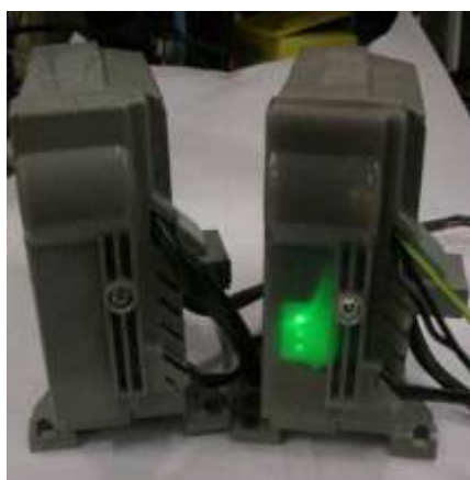
Fig. 8.2.1/ 1 Inverter with diagnostic LED
