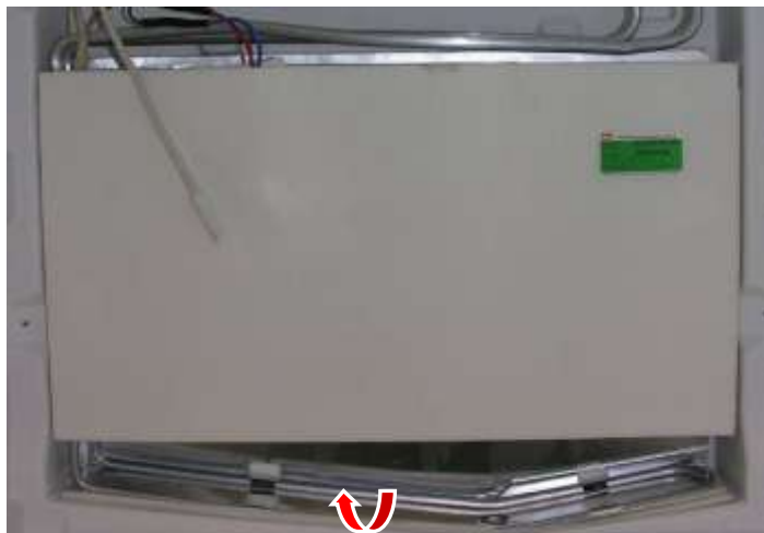
Fig. 5.3.1/ 2 Swinging out the evaporator module
